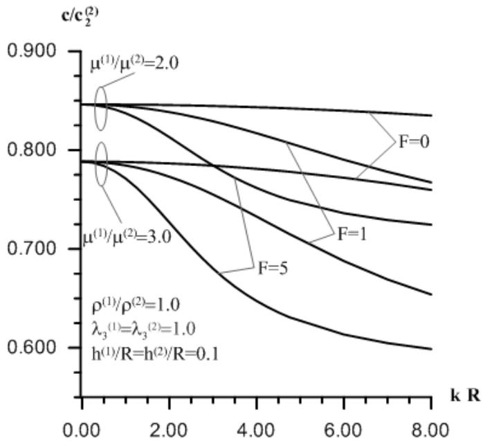
Figure 4. The influence of the parameter  $F$  on dispersion curves under higher values of  $\mu^{(1)}/\mu^{(2)}$ .
