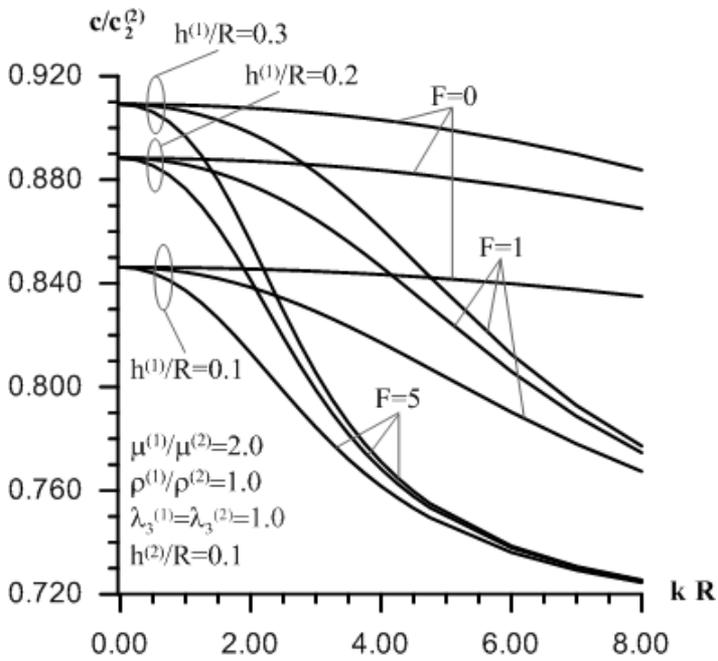
**Figure 2.** The influence of the parameter  $F$  on dispersion curves under various  $h^{(1)}/R$ .
