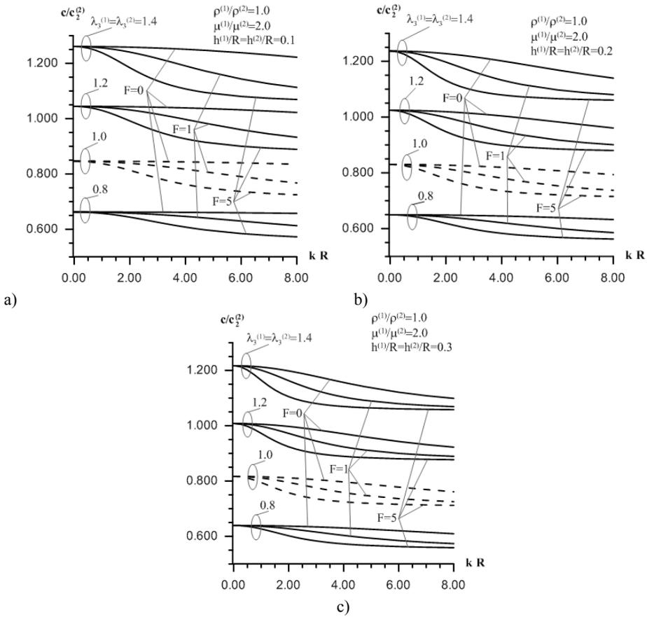
**Figure 6.** The influence of the parameter  $F$  on dispersion curves under various values of the initial strains. a)  $h^{(1)}/R = h^{(2)}/R = 0.1$  b)  $h^{(1)}/R = h^{(2)}/R = 0.2$  c)  $h^{(1)}/R = h^{(2)}/R = 0.3$
