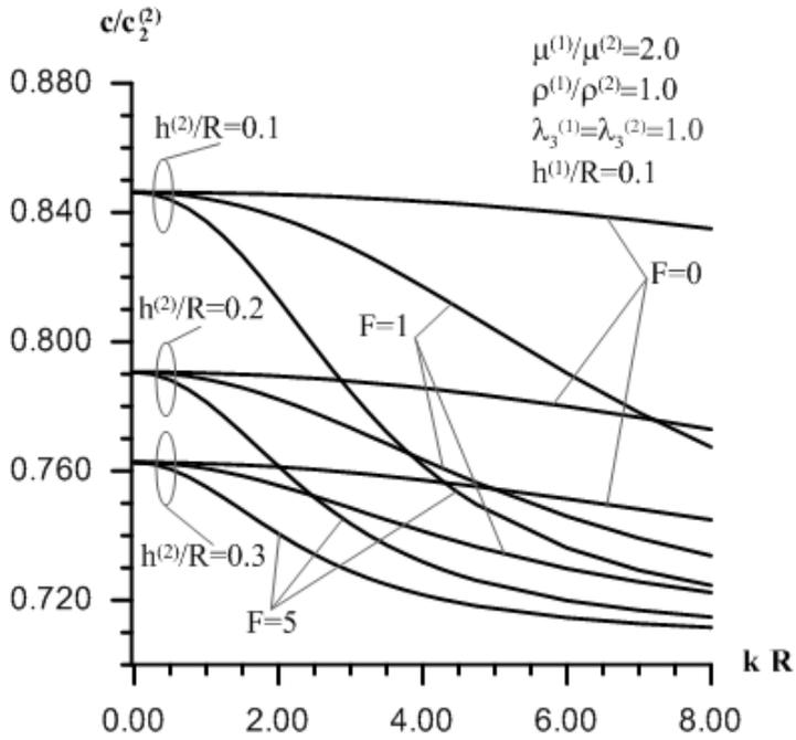
Figure 3. The influence of the parameter  $F$  on dispersion curves under various  $h^{(2)}/R$ .
