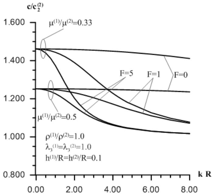
**Figure 5.** The influence of the parameter  $F$  on dispersion curves under lower varies  $\mu^{(1)} / \mu^{(2)}$ .
