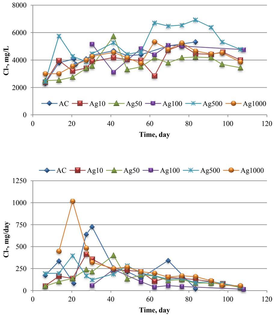
Figure 3. Variations of chloride values of leachate in all bioreactors
