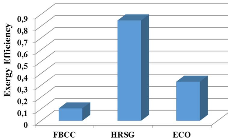
Figure 5. Exergetic efficiency for the major components
