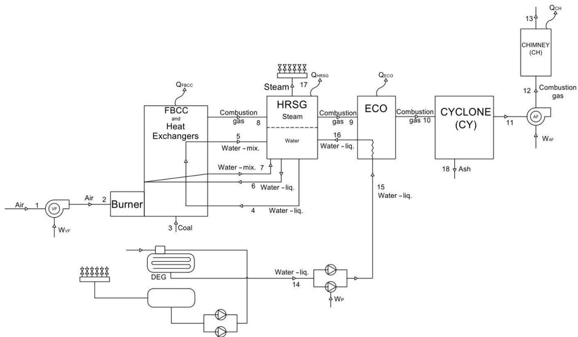
**Figure 1.** Schematic diagram of the power plant [10]
