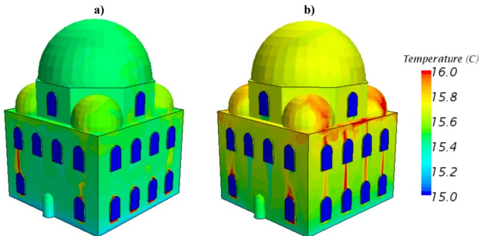
**Figure 4.** The temperature distributions at the inner surface of the walls at the end of **a)** 3600 s and **b)** 5400 s.
