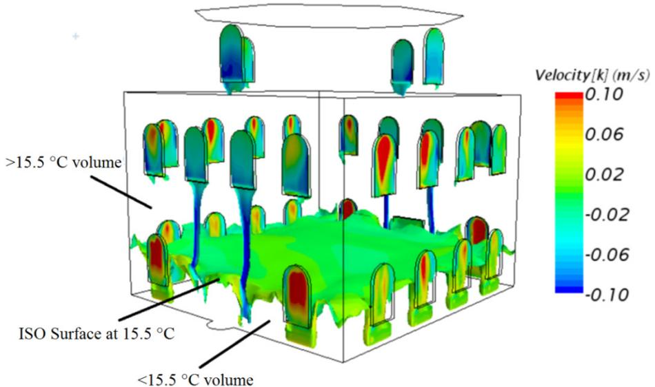
**Figure 7.** Velocity gradients on the ISO surface in a vertical direction at 15.5 °C after 5400 seconds. Positive and negative values indicate that the velocity vectors are up and down, respectively.
