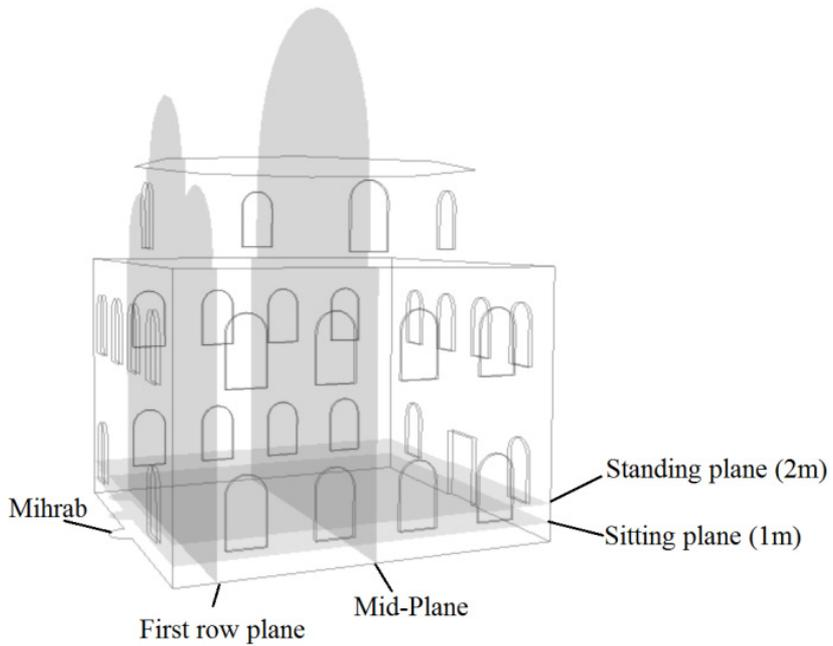
**Figure 2. Planes on the models used to analyze temperature distribution.**
