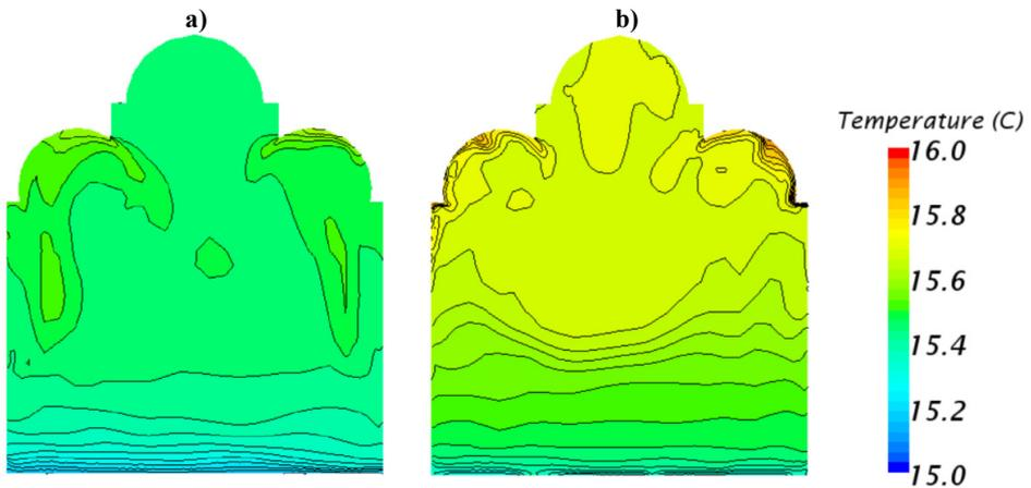
**Figure 6.** The temperature distribution at the end of the **a)** 3600 s and **b)** 5400 s on the first plane.
