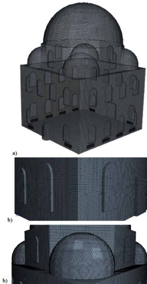
**Figure 3. a)** The transparent appearance of the mesh, **b)** the mesh of the small domes and walls.
