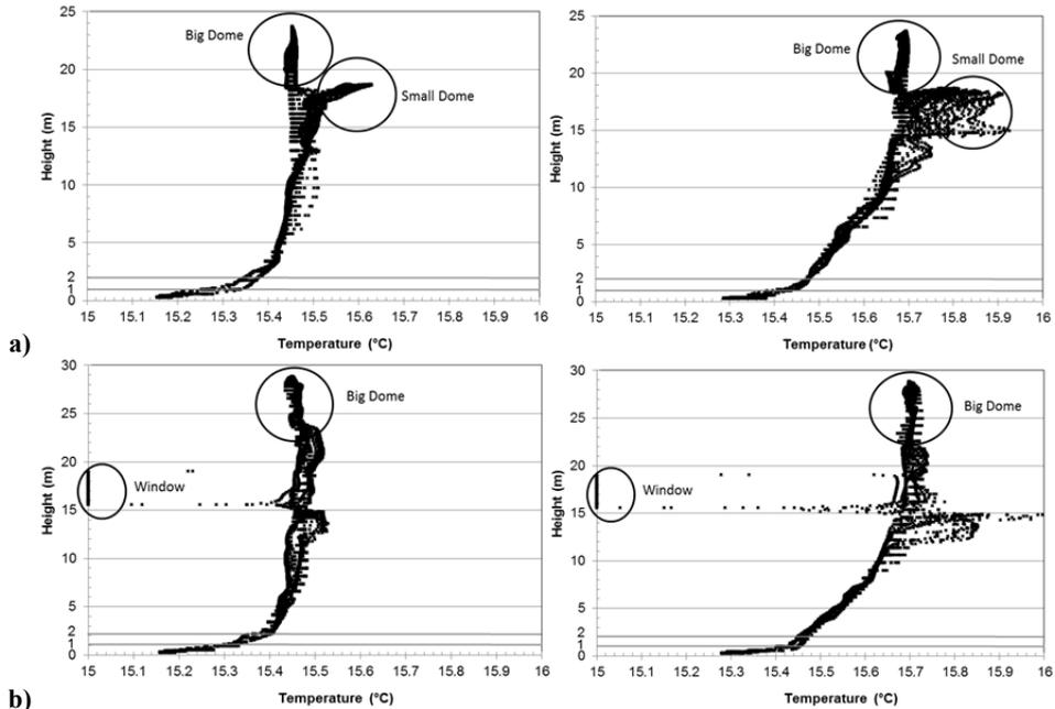
**Figure 5.** The temperature distribution at the end of the 3600 s and 5400 s in the a) first plane and b) mid-plane.
