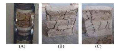
Fig. 4. Failure pattern under compressive loads
