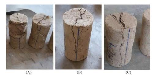
Fig. 5. Failure pattern under tensile loads
