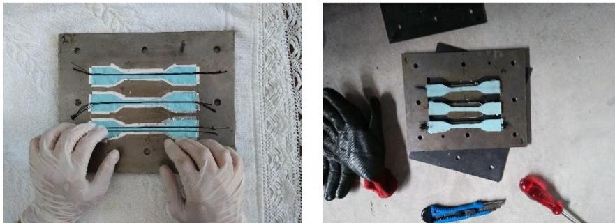
**Figure 7.** Preparation of specimen, die and specimens
