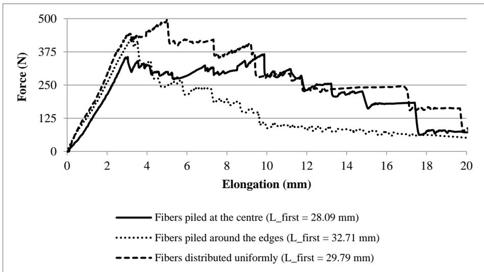
**Figure 18.** The force-elongation diagram of the rubber composite with no-slippage fibers as Nylon 6.6 in various conditions
