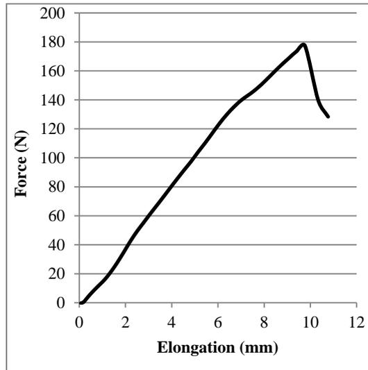
**Figure 2.** Tensile test results where the fibers are two-layered and uniformly distributed (angle is  $0^\circ$  between fibers)
