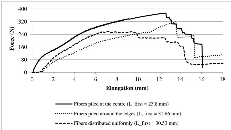
**Figure 16.** The force-elongation diagram of the rubber composite with no-slippage fibers as Polyester no:50 in various conditions
