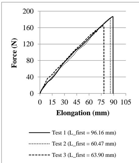
**Figure 11.** Nylon 6.6 cord tensile tests, force-elongation diagram
