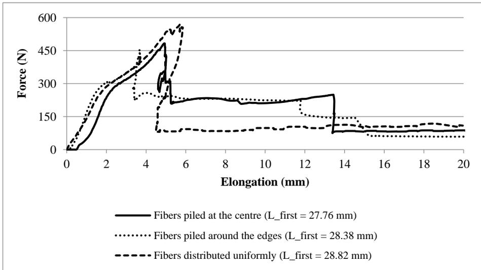
**Figure 17.** The force-elongation diagram of the rubber composite with no-slippage fibers as Polyester no:20 in various conditions
