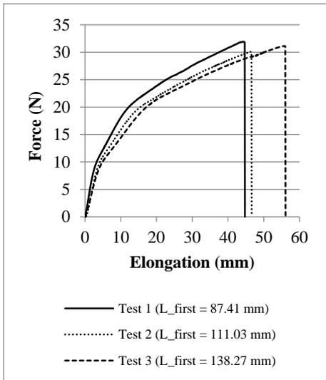
**Figure 9.** Polyester no:50 cord tensile tests, force-elongation diagram
