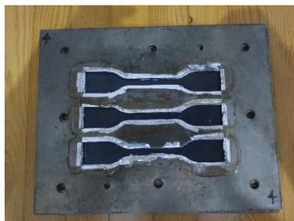
Figure 5. Specimen preparation die
