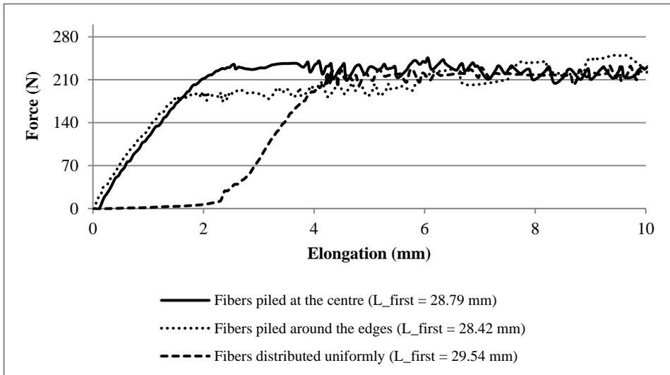
**Figure 15.** The force-elongation diagram of the rubber composite with slippage fibers as Nylon 6.6 in various conditions
