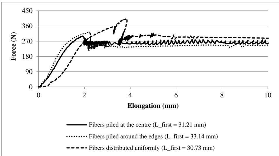
**Figure 14.** The force-elongation diagram of the rubber composite with slippage fibers as Polyester no:20 in various conditions
