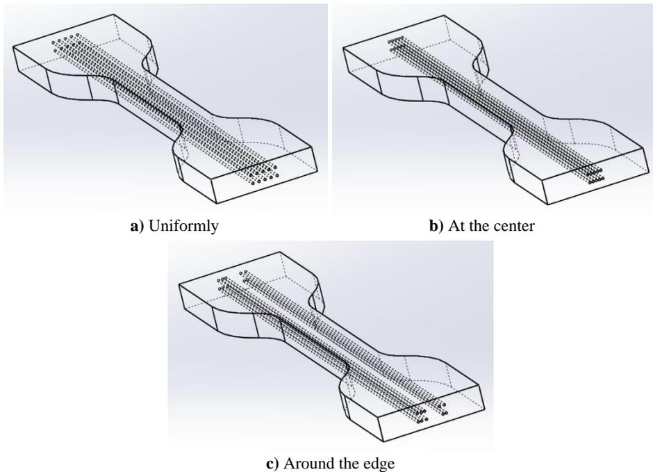
**Figure 3.** a) Uniformly, b) at the center and c) around the edge distributed fiber-reinforced rubber specimen model (angle is  $0^\circ$  between fibers)
