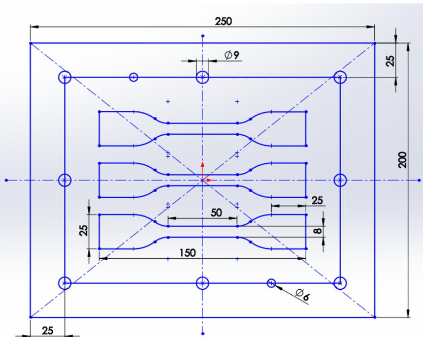
Figure 4. The technical drawing of the die
