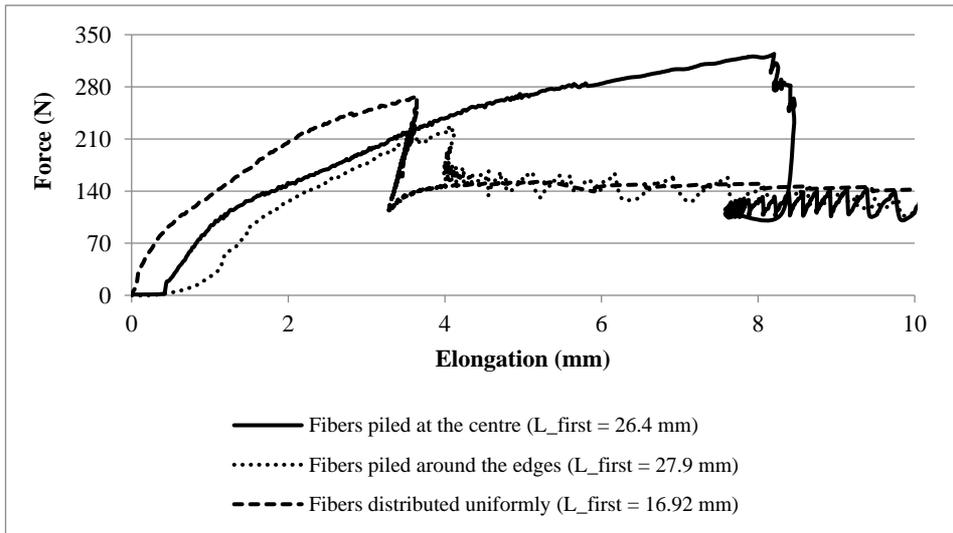
**Figure 13.** The force-elongation diagram of the rubber composite with slippage fibers as Polyester no:50 in various conditions
