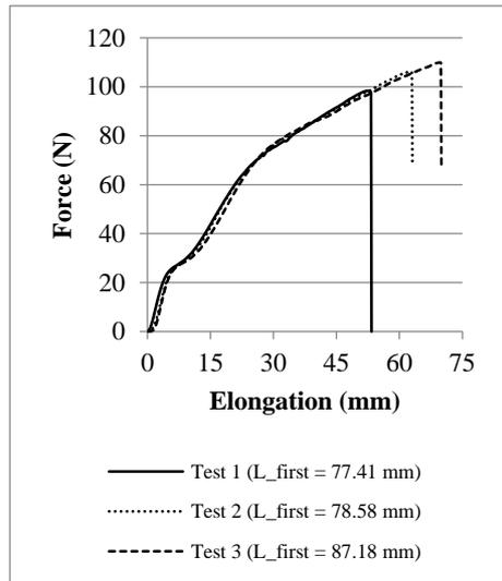
**Figure 10.** Polyester no:20 cord tensile tests, force-elongation diagram
