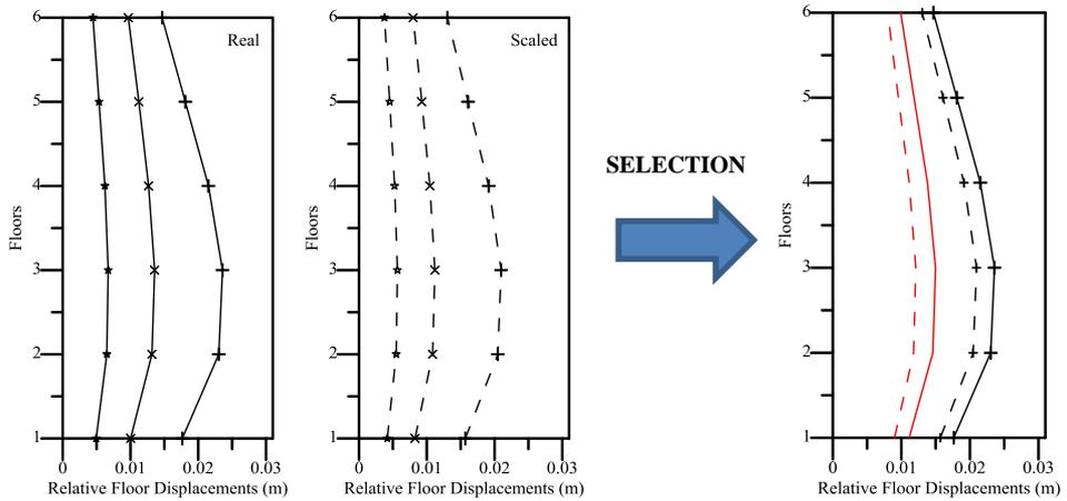
**Figure 28.** Relative floor displacement for group 15 records (P0530-P0745-P0810)
