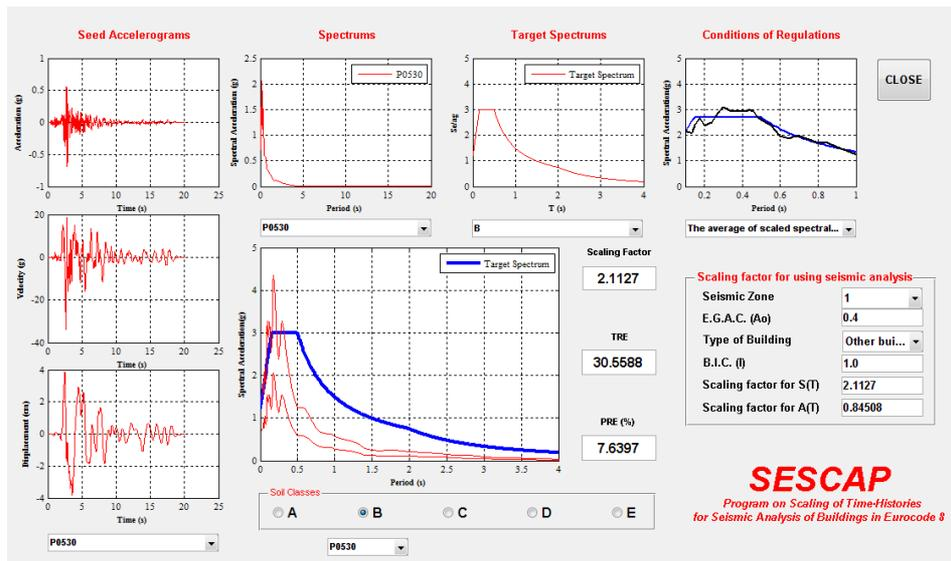
Figure 9. Scaling Results of N. Palm Springs Earthquake
