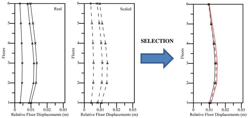
**Figure 45.** Relative floor displacement for group 32 records (P1109-P0865-P0745)
