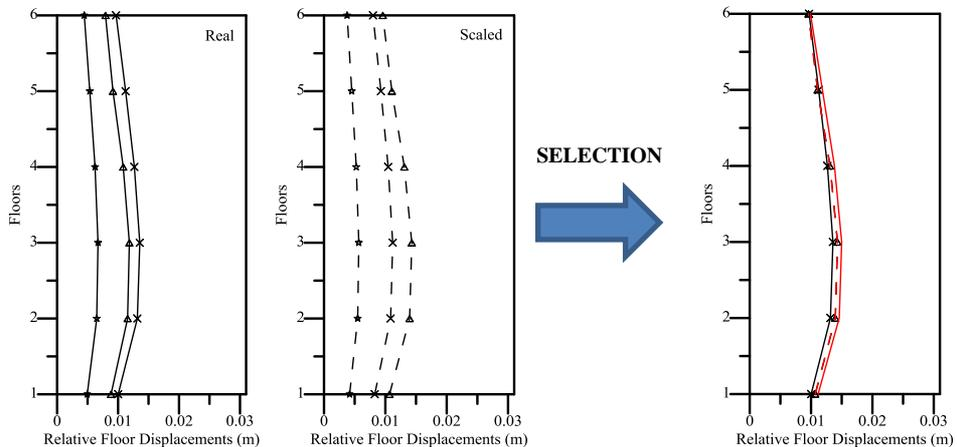
**Figure 48.** Relative floor displacement for group 35 records (P0530-P0865-P0745)
