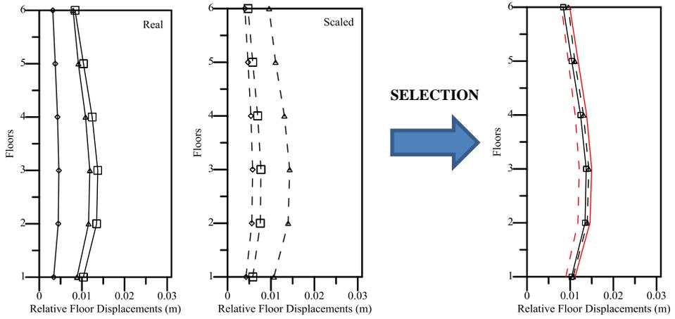
**Figure 33.** Relative floor displacement for group 20 records (P1109-P0865-P1169)
