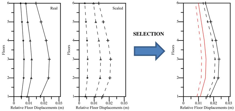
**Figure 27.** Relative floor displacement for group 14 records (P0530-P0865-P0810)
