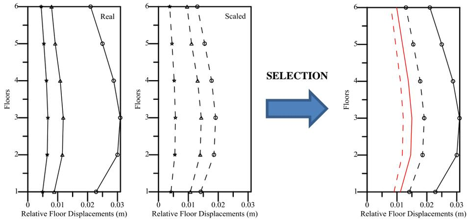
**Figure 43.** Relative floor displacement for group 30 records (P0530-P0865-P1043)
