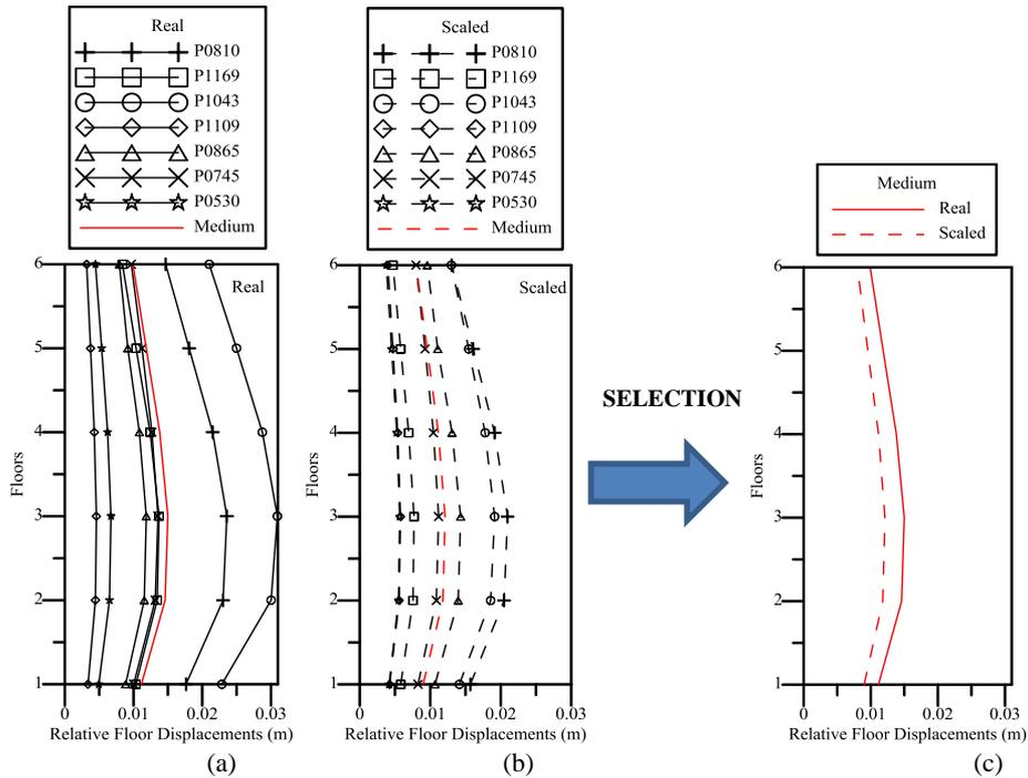
**Figure 13.** Relative floor displacement for real, scaled seven records and mean of them
