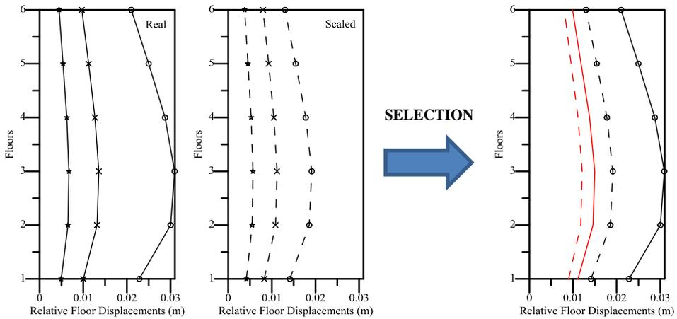
**Figure 44.** Relative floor displacement for group 31 records (P0530-P0745-P1043)
