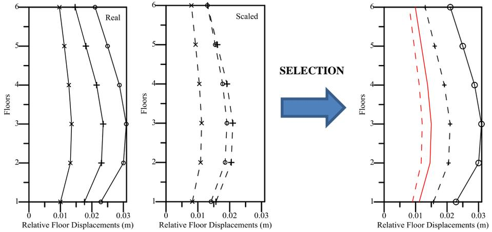
**Figure 21.** Relative floor displacement for group 8 records (P0745-P0810-P1043)
