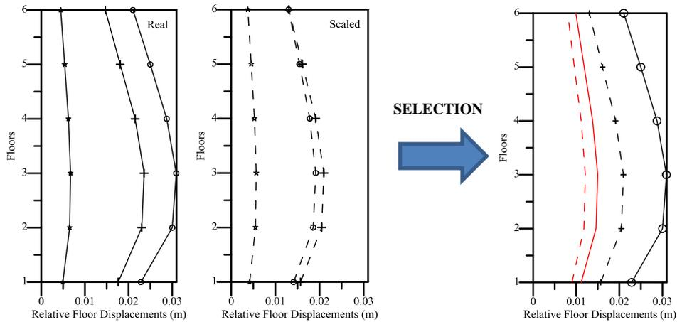
**Figure 22.** Relative floor displacement for group 9 records (P0530-P0810-P1043)
