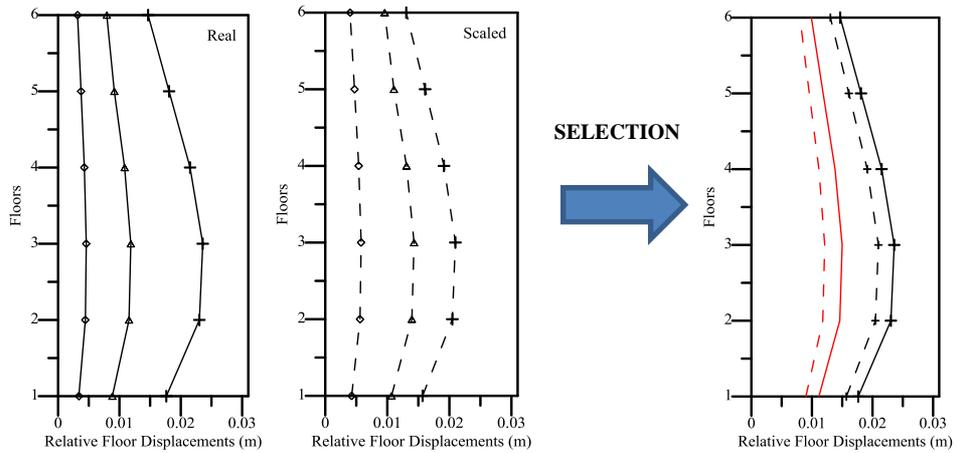
**Figure 23.** Relative floor displacement for group 10 records (P1109-P0865-P0810)
