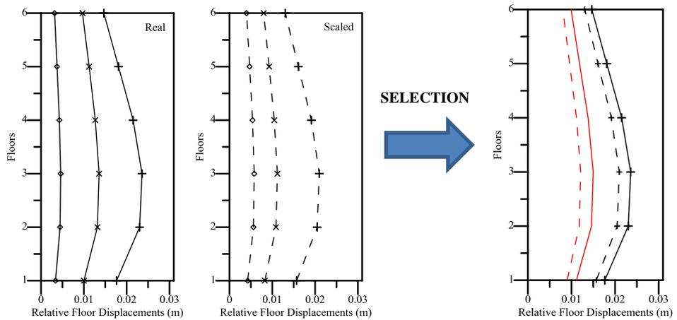
**Figure 24.** Relative floor displacement for group 11 records (P1109-P0745-P0810)
