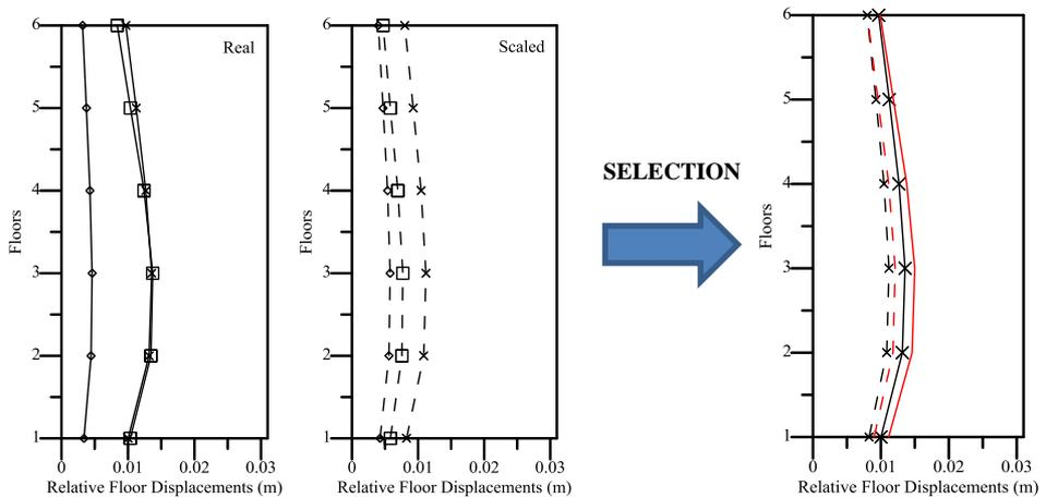
**Figure 34.** Relative floor displacements for group 21 records (P1109-P1169-P0745)
