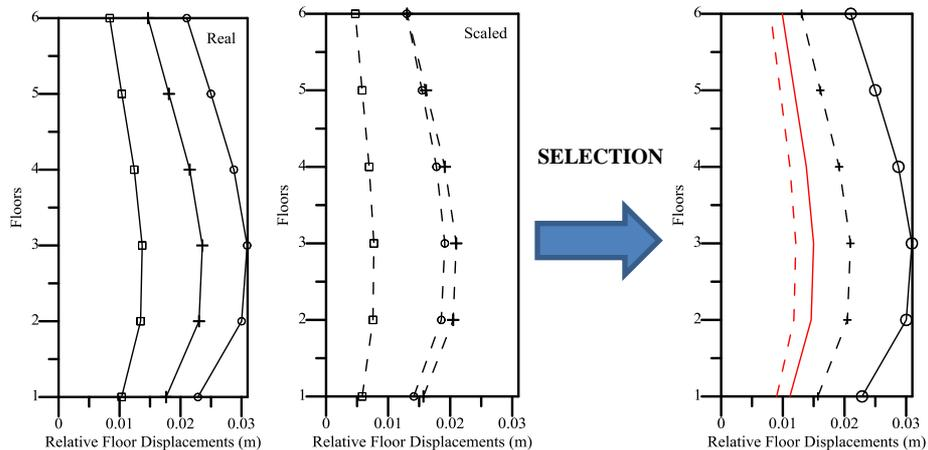
**Figure 14.** Relative floor displacement for group1 records (P1169-P0810-P1043)
