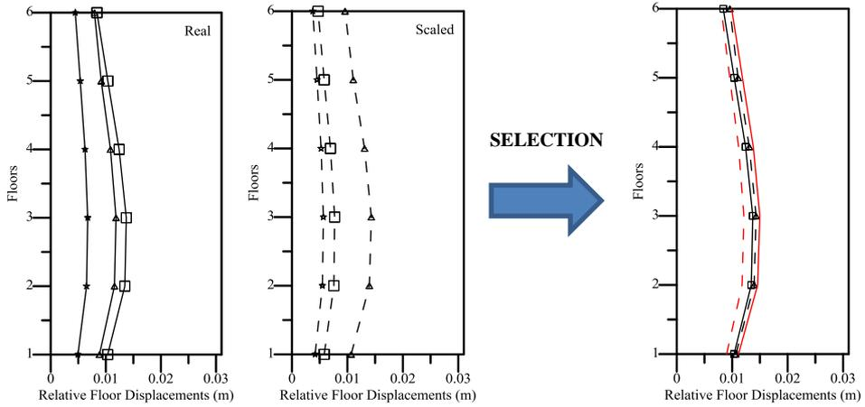
**Figure 37.** Relative floor displacement for group 24 records (P0530-P0865-P1169)
