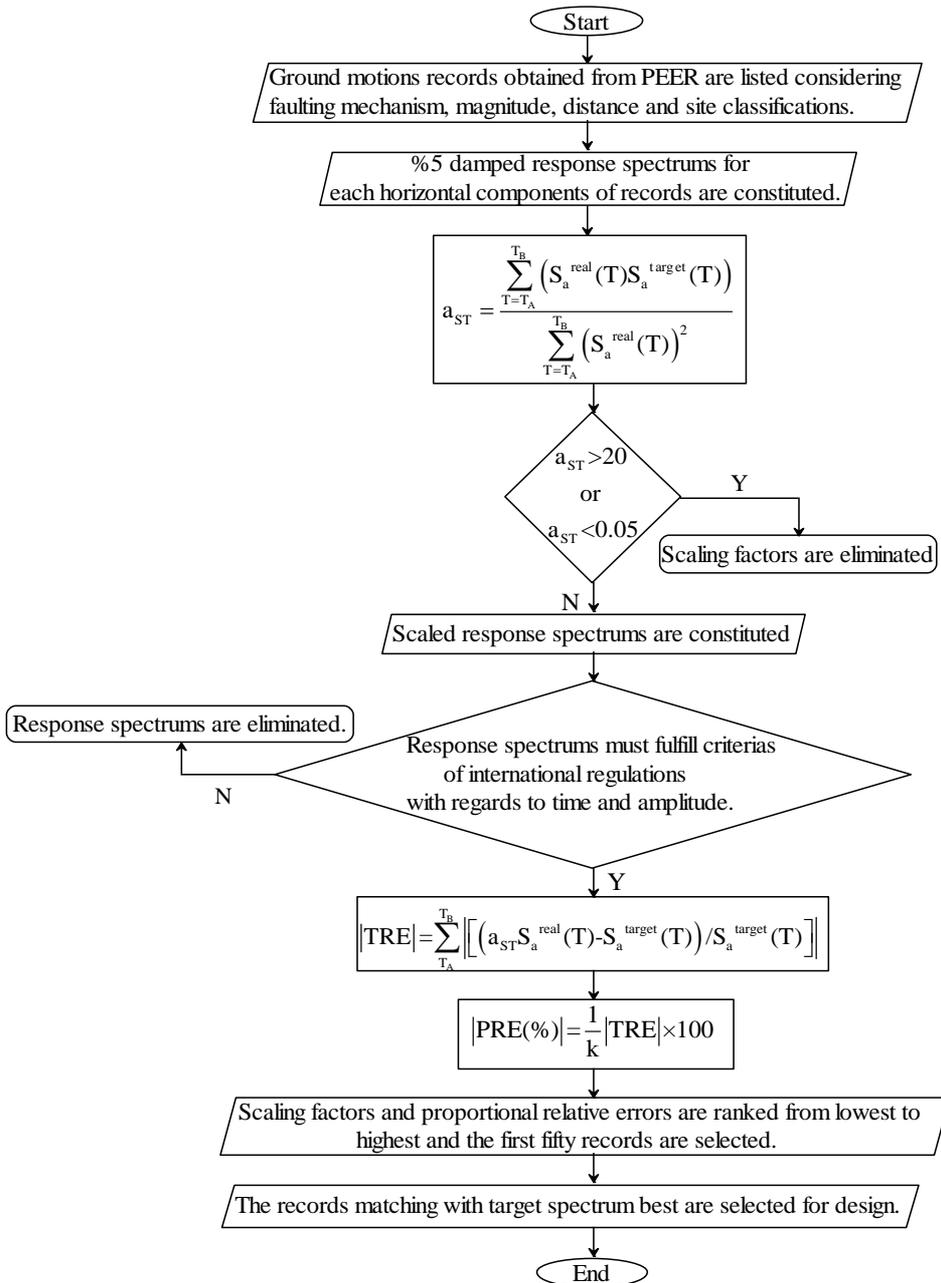
Figure 1. Flow chart diagram of time domain method
