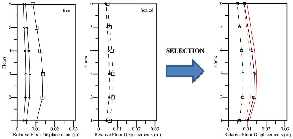
**Figure 35.** Relative floor displacement for group 22 records (P1109-P0530-P1169)
