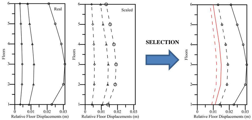
**Figure 39.** Relative floor displacement for group 26 records (P1109-P0865-P1043)
