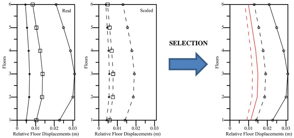
**Figure 32.** Relative floor displacement for group 19 records (P0530-P1169-P1043)
