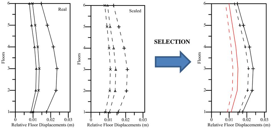
**Figure 26.** Relative floor displacement for group 13 records (P0865-P0745-P0810)
