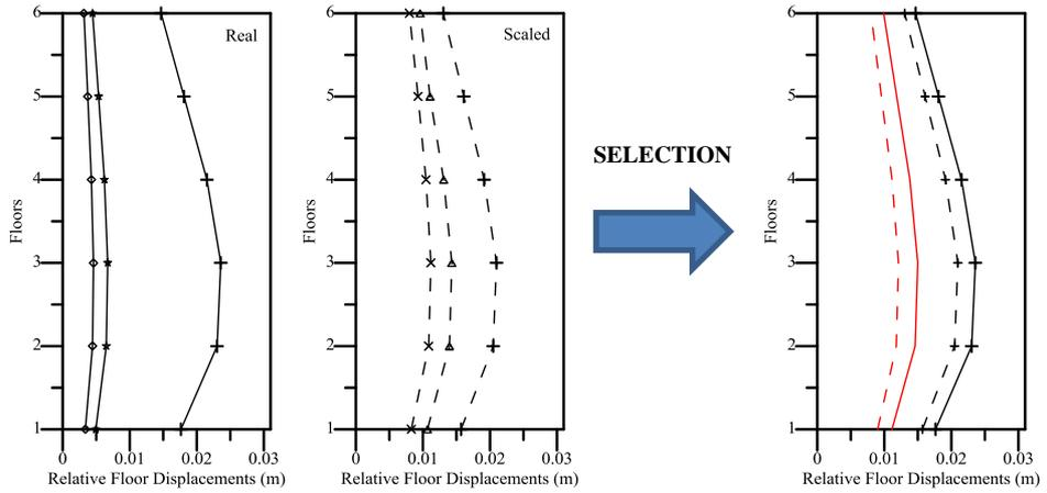
**Figure 25.** Relative floor displacement for group 12 records (P1109-P0530-P0810)
