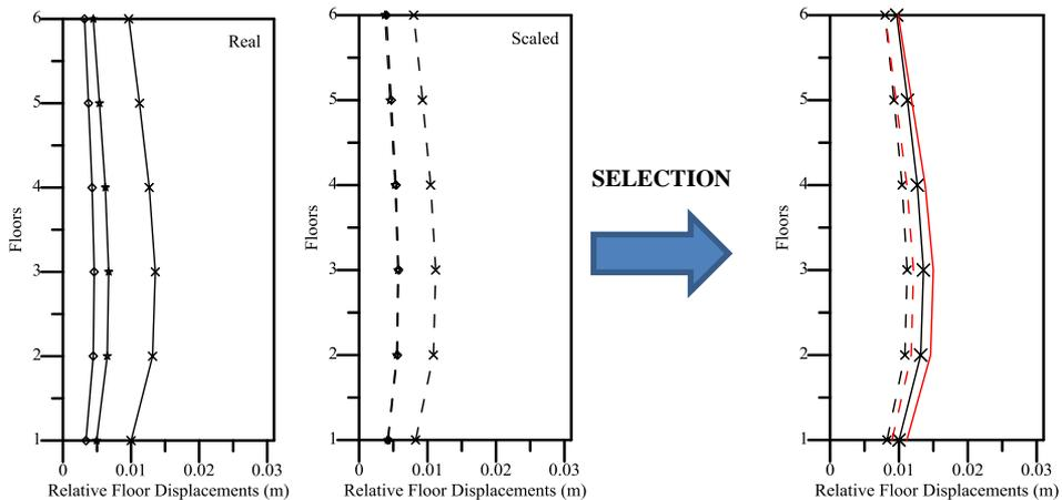
**Figure 47.** Relative floor displacement for group 34 records (P1109-P0530-P0745)
