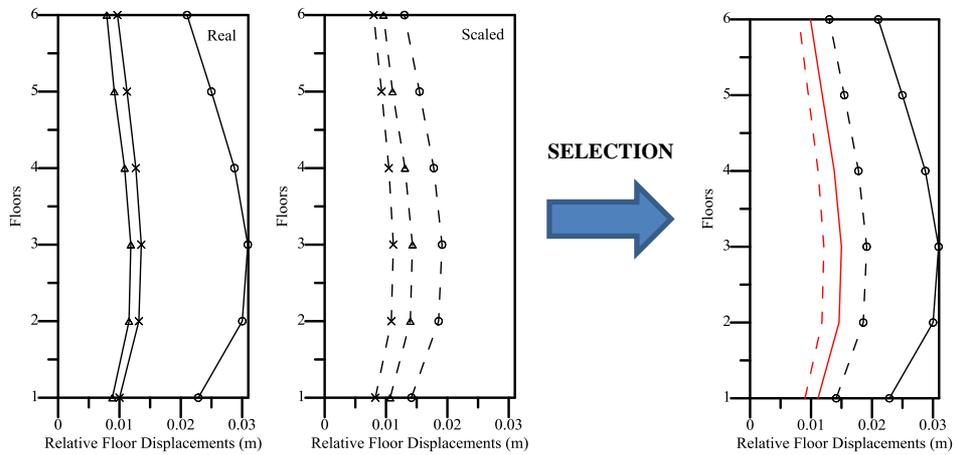
**Figure 42.** Relative floor displacement for group 29 records (P0865-P0745-P1043)
