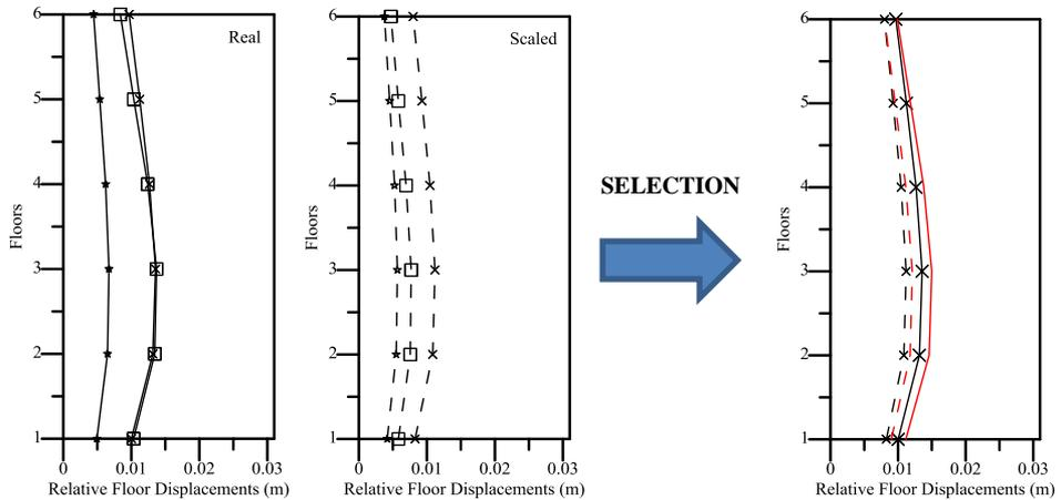
**Figure 38.** Relative floor displacement for group 25 records (P0530-P1169-P0745)
