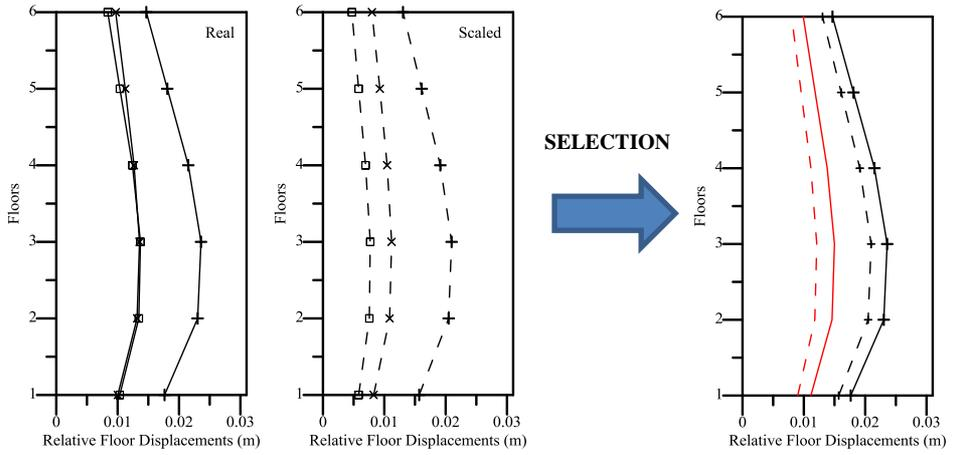
Figure 17. Relative floor displacement for group 4 records (P1169-P0745-P0810)
