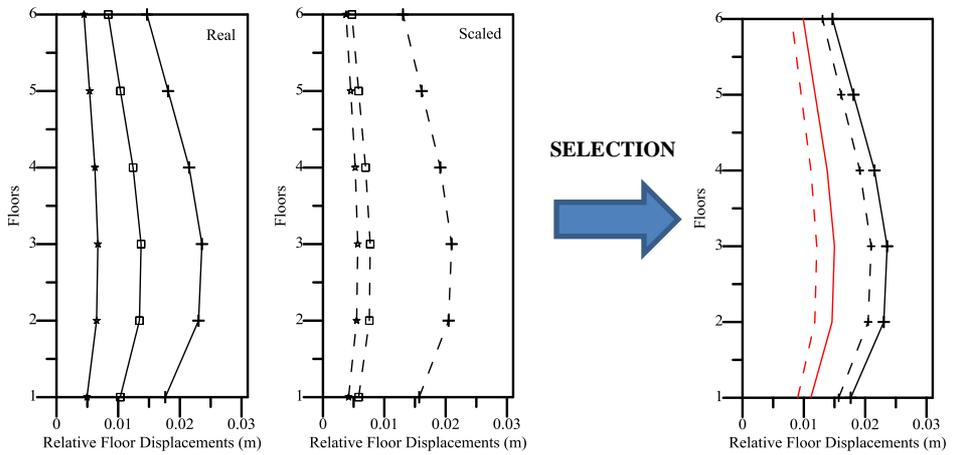
Figure 18. Relative floor displacement for group 5 records (P0530-P1169-P0810)
