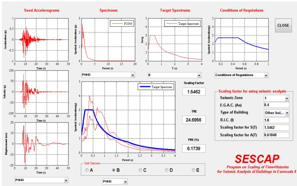
Figure 5. Scaling Results of Kobe Earthquake
