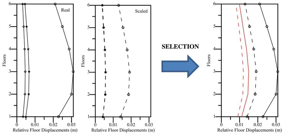
**Figure 41.** Relative floor displacement for group 28 records (P1109-P0530-P1043)
