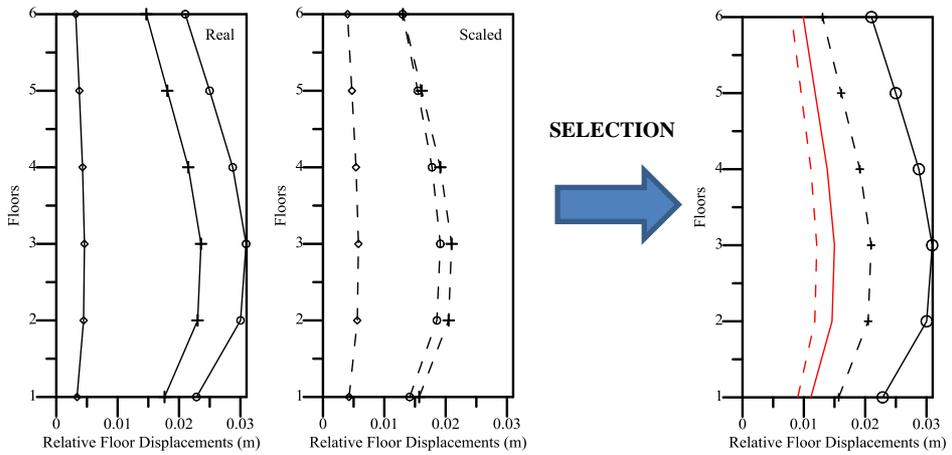
**Figure 19.** Relative floor displacement for group 6 records (P1109-P0810-P1043)
