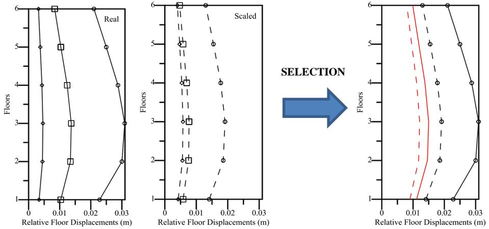
**Figure 29.** Relative floor displacement for group 16 records (P1109-P1169-P1043)
