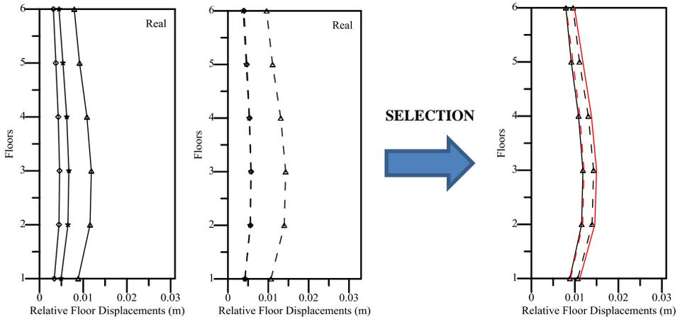
**Figure 46.** Relative floor displacement for group 33 records (P1109-P0530-P0865)
