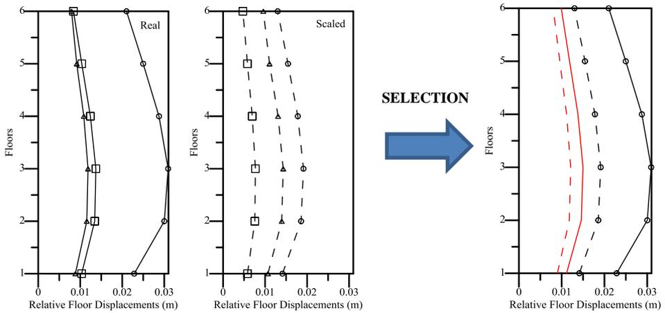
**Figure 30.** Relative floor displacement for group 17 records (P0865-P1169-P1043)
