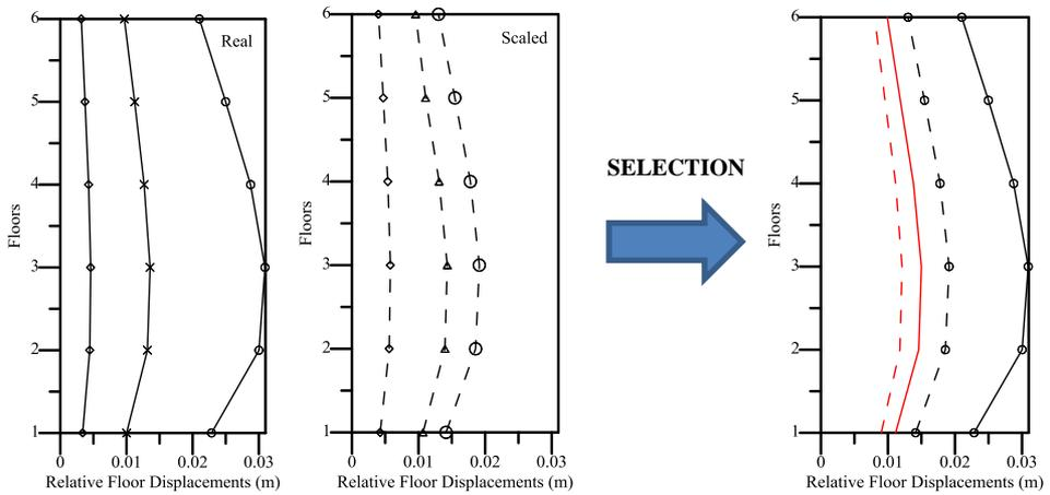
**Figure 40.** Relative floor displacement for group 27 records (P1109-P0745-P1043)
