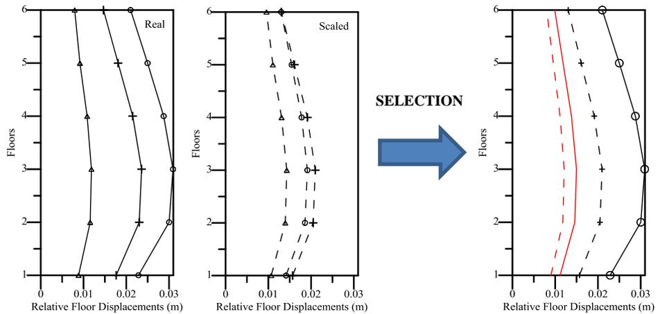
**Figure 20.** Relative floor displacement for group 7 records (P0865-P0810-P1043)
