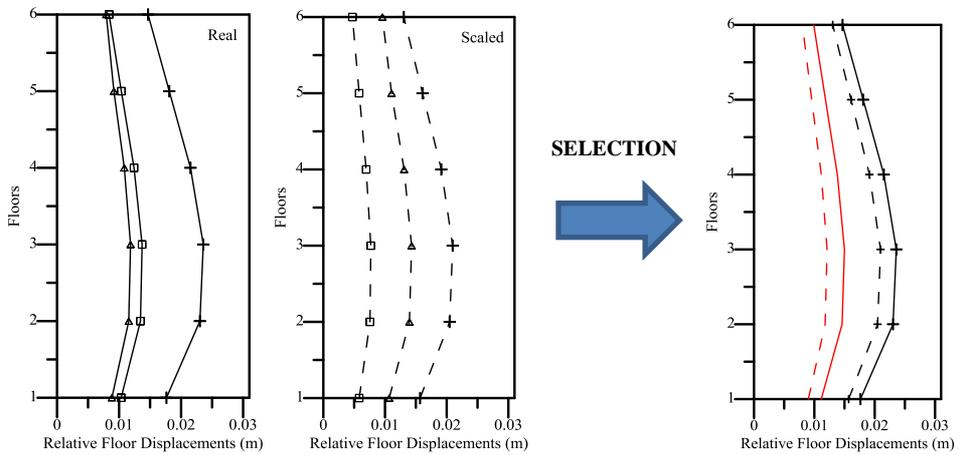
**Figure 16.** Relative floor displacement for group 3 records (P0865-P1169-P0810)
