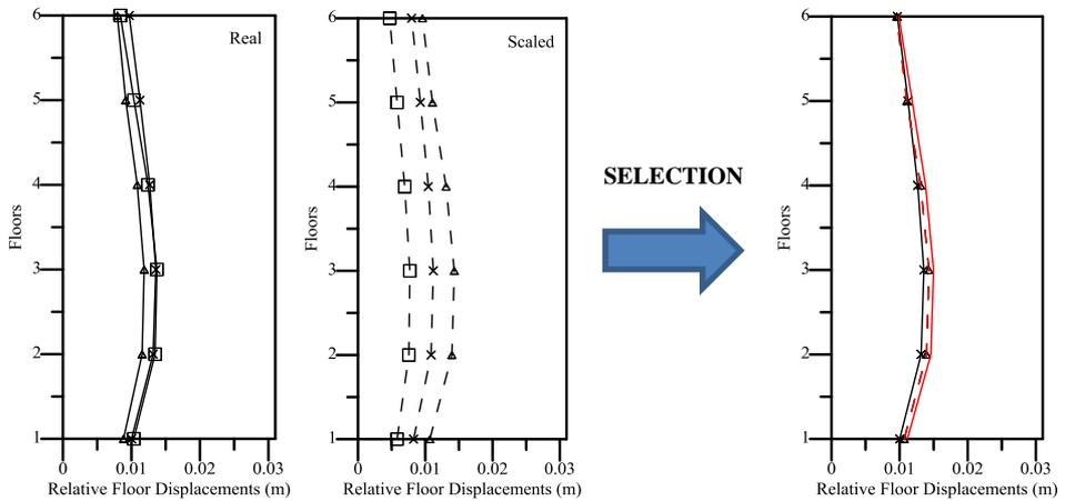
**Figure 36.** Relative floor displacement for group 23 records (P0865-P1169-P0745)
