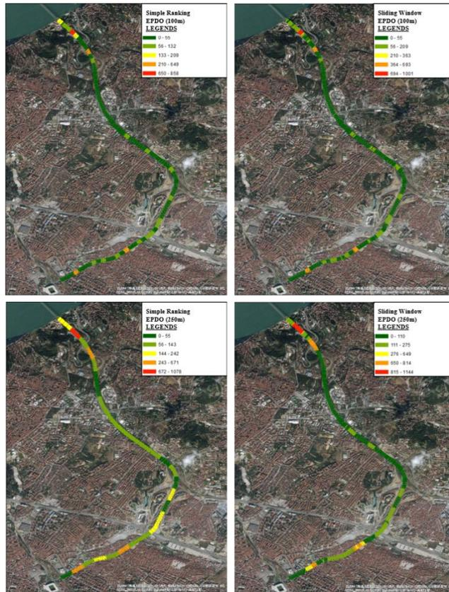
Figure 8. Application of simple ranking and sliding window methods for EPDO-ACF
