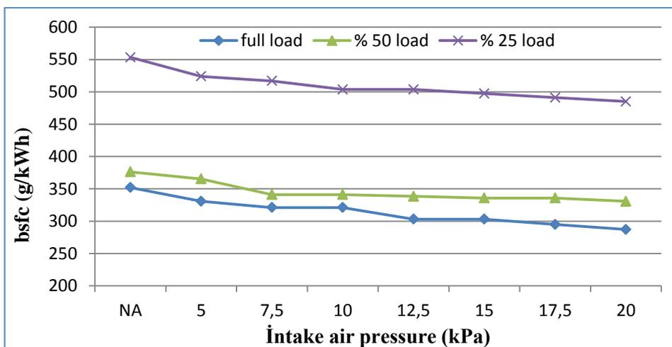
**Figure 2.** Variation of brake specific fuel consumption (bsfc)
