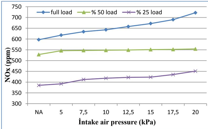
**Figure 8.** Change in  $\text{NO}_x$  amount depending on engine intake air pressure increase.
