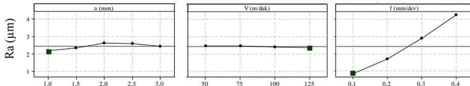
**Figure 3.** The effect of cutting parameters on means response characteristics for surface roughness.
