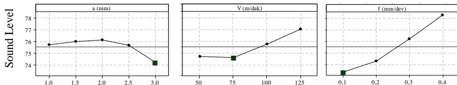
**Figure 7.** The effect of cutting parameters on means response characteristics for sound level.
