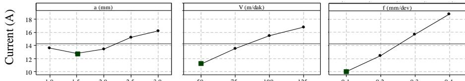
**Figure 9.** The effect of cutting parameters on means response characteristics for motor current.
