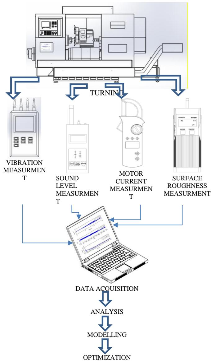
**Figure 2.** Schematic view of the experimental set-up.
