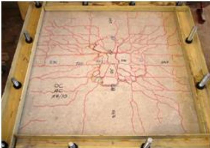
**Figure 18.** Failure pattern of AGB4 slab
