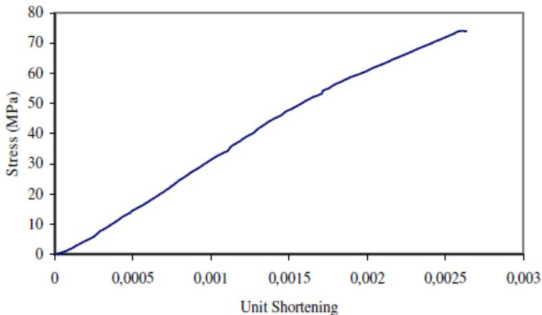
**Figure 1.** Stress-Strain curve for high-strength concrete
