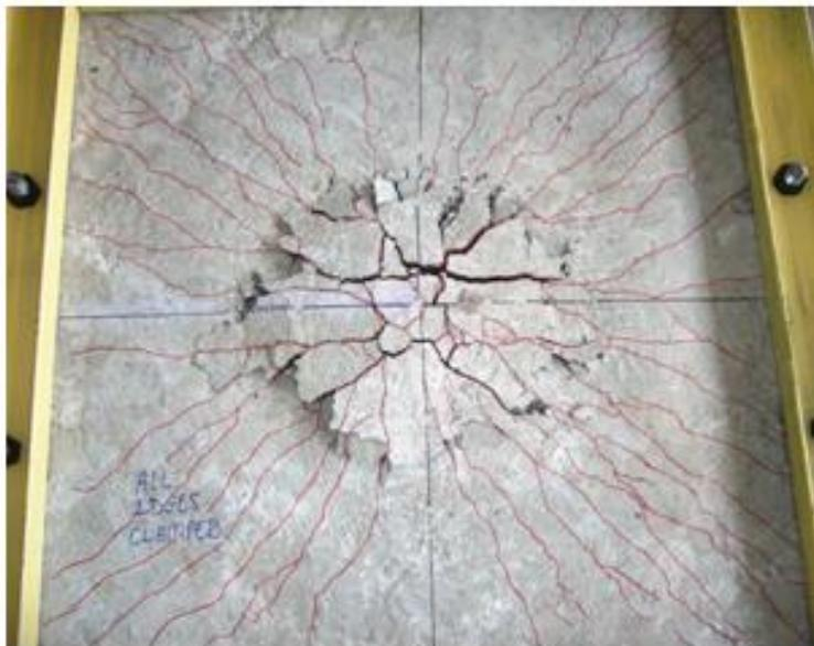
Figure 12. Failure pattern of AB4 slab
