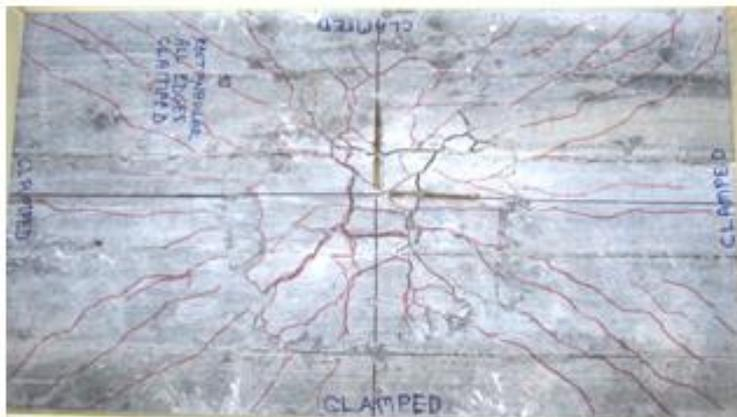
Figure 10. Failure pattern of AD4 slab
