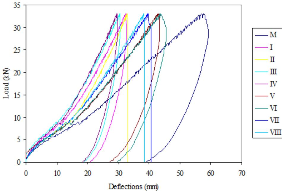
**Figure 17.** Load Deflection curve of AGB4 slab
