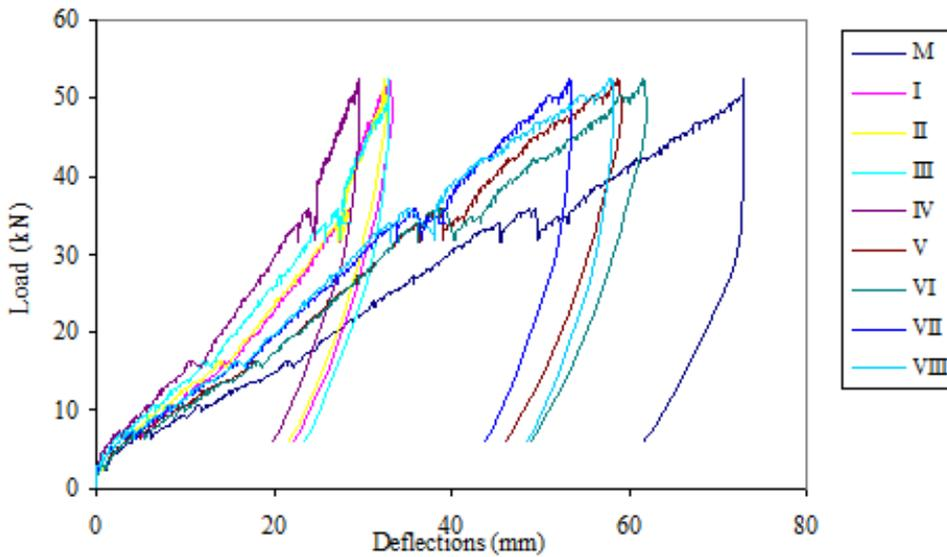
Figure 11. Load Deflection curve of AB4 slab
