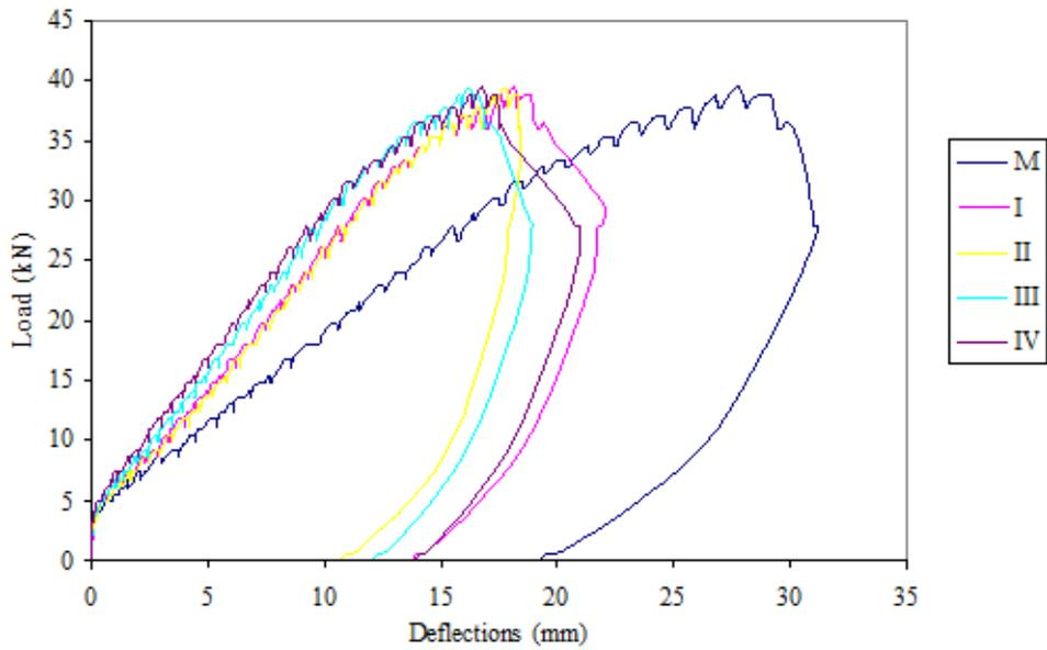
Figure 13. Load Deflection curve of AG4 slab
