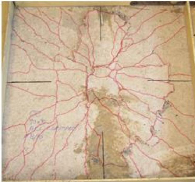
Figure 14. Failure pattern of AG4 slab
