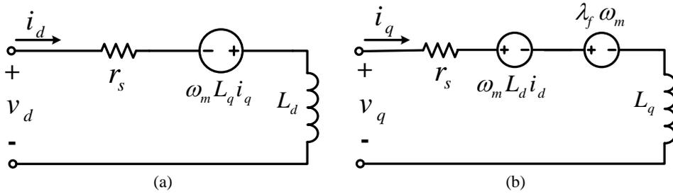
Figure 3. PMSM equivalent circuit model: a) d-axis, b) q-axis
