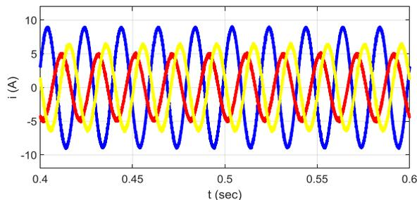
**Figure 17.** Inverter output current at unbalance load scenario
