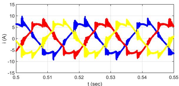
**Figure 20.** Inverter output current at nonlinear load scenario
