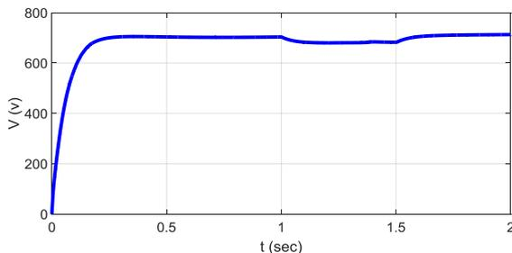
**Figure 12.** DC-link voltage at variable load scenario
