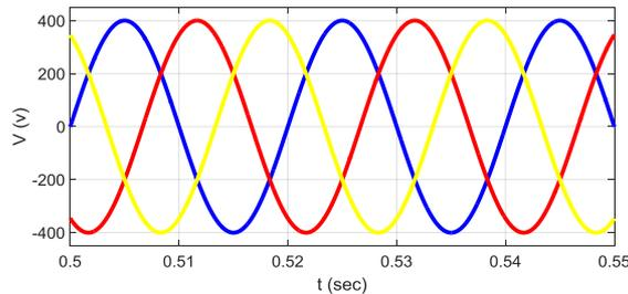
**Figure 15.** Output voltage at unbalance load scenario
