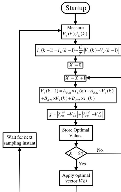
Figure 6. MPC flowchart based on voltage control
