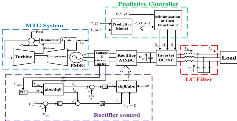
Figure 1. The MTG system controlled by MPC
