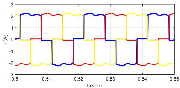
**Figure 19.** Output current at nonlinear load scenario
