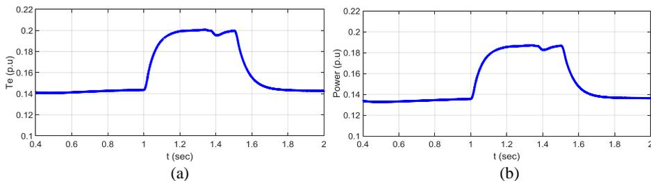
**Figure 14.** (a) PMSG electromagnetic torque, (b) PMSG active power at variable load scenario
