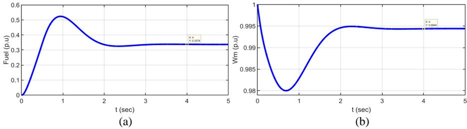
**Figure 8.** (a) Fuel demand signal, (b) MT output speed at constant load scenario
