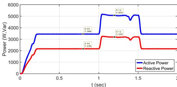
**Figure 13.** Output power at variable load scenario
