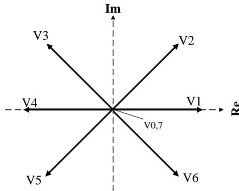
**Figure 5.** Generated voltage vectors of inverter across complex plane
