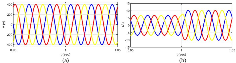
**Figure 11.** (a) Output voltage, (b) output current at variable load scenario
