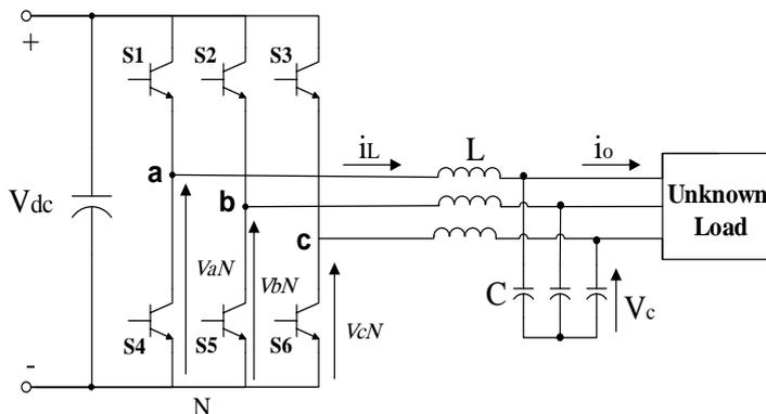
**Figure 4.** Three-phase inverter with LC filter and unknown load
