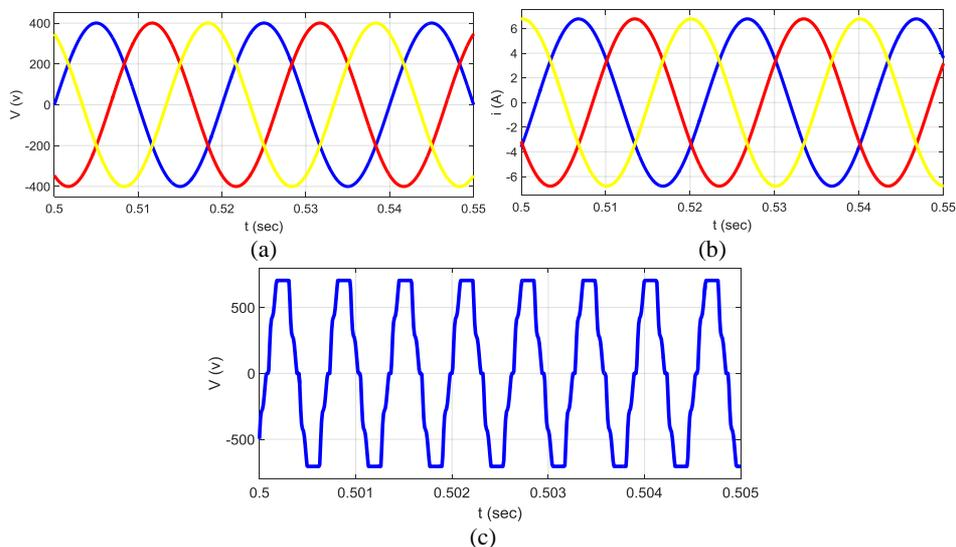
**Figure 7.** (a) Output voltage, (b) output current, (c) PMSG output voltage at constant load scenario
