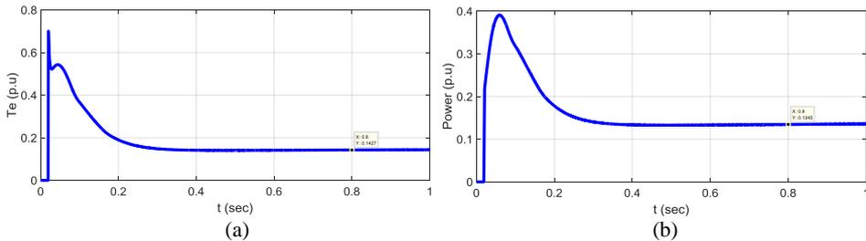
**Figure 10.** (a) PMSG electromagnetic torque, (b) PMSG active power at constant load scenario
