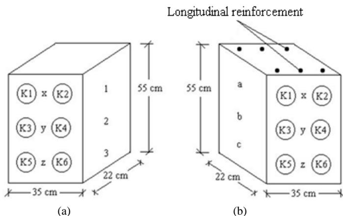
**Figure 1.** Test locations on (a) concrete and (b) reinforced concrete members.
