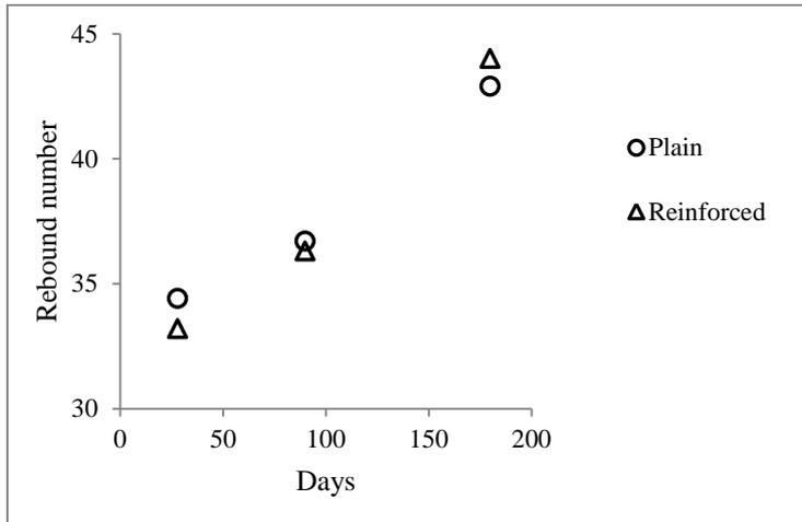
Figure 5. RH test results of plain concrete and reinforced concrete members
