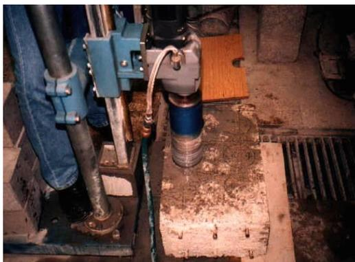
**Figure 2.** Extraction of core specimens from the members
