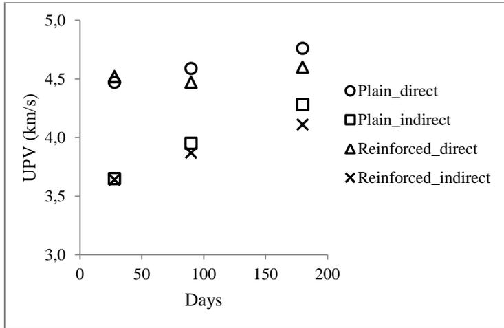
Figure 4. UPV test results of plain concrete and reinforced concrete members
