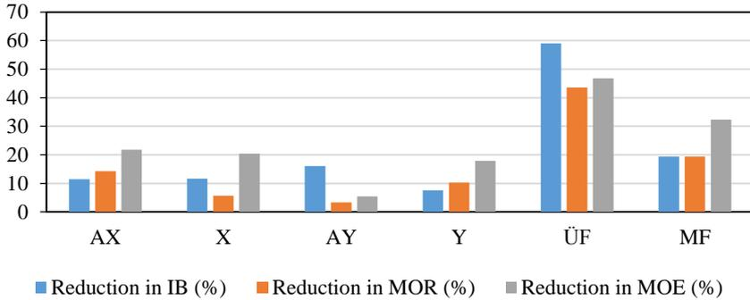
**Figure 1.** Changes in mechanical strengths of experimental panels after weathering
