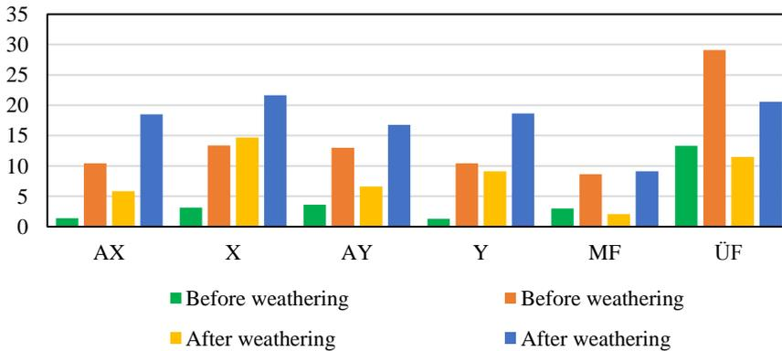
**Figure 2.** Changes in thickness swelling of experimental panels after weathering
