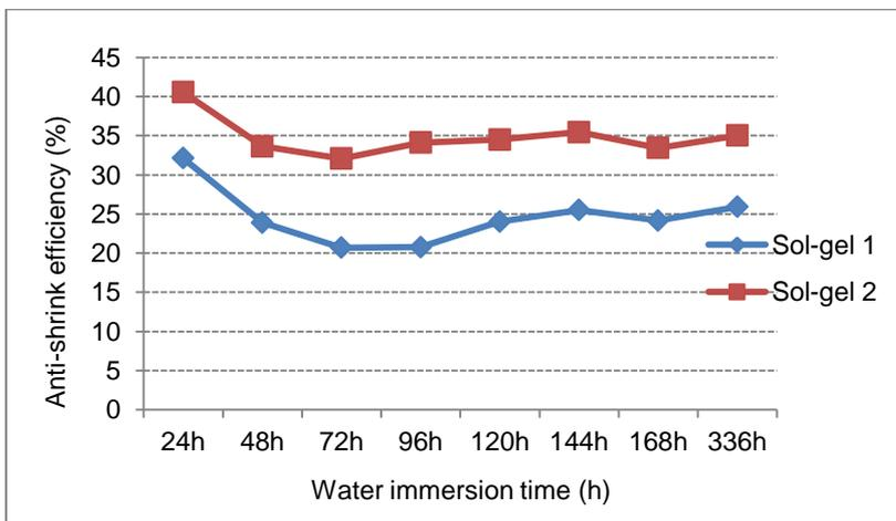
**Figure 2.** Anti-shrink efficiency of specimens during 14 days of water immersion
