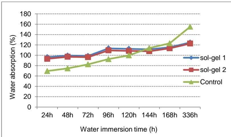
**Figure 1.** Water absorption of specimens during 14 days of water immersion
