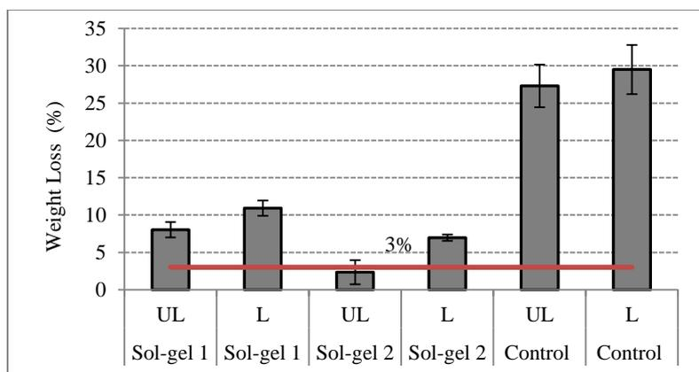
**Figure 3.** Weight loss of decayed specimens by *C. puteana*
