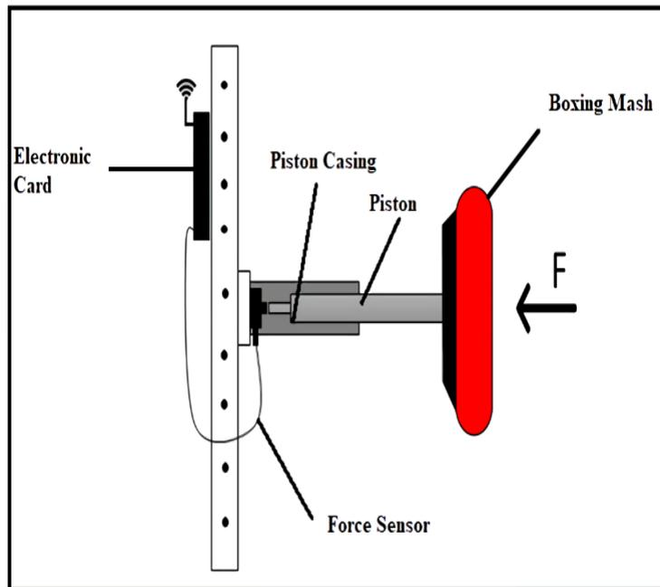
Figure 2. The basic unit of measurement that forms the training measurement system.
