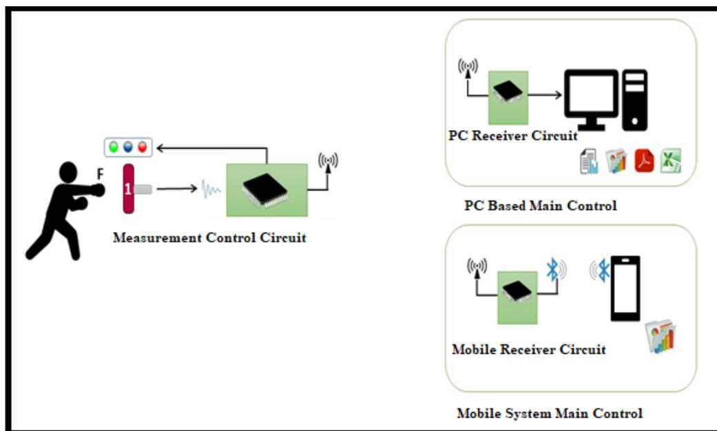
Figure 1. Hardware block diagram of the training measurement system.
