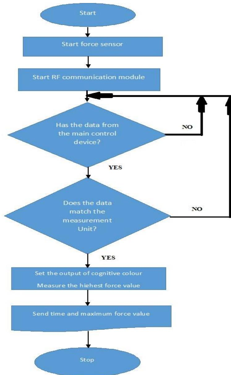
**Figure 6.** Software algorithm of the training measurement system.
