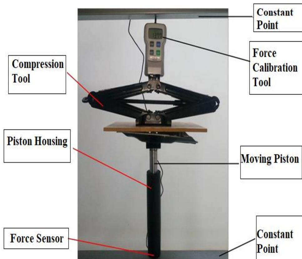
**Figure 4.** Test setup for force measurement calibration.
