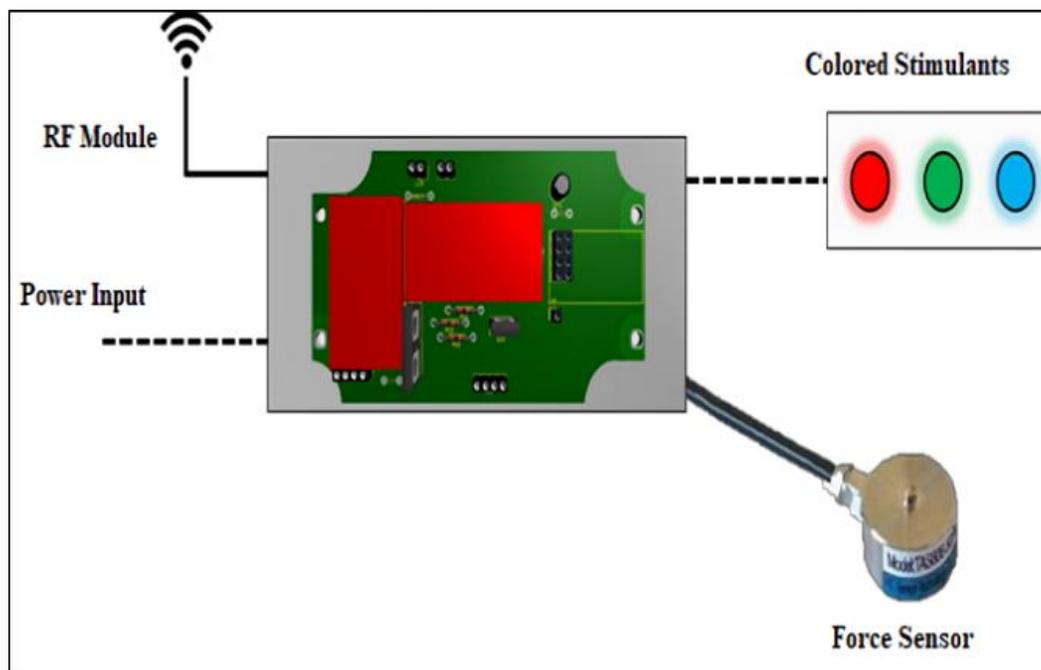
Figure 3. Electronic design of the basic measurement unit.
