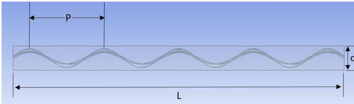
**Figure 2.** Wire coil inserted in a square duct.
