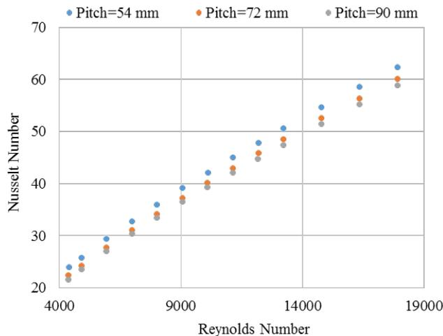
**Figure 10.** Results of Nusselt number versus Reynolds number for DWC insert.
