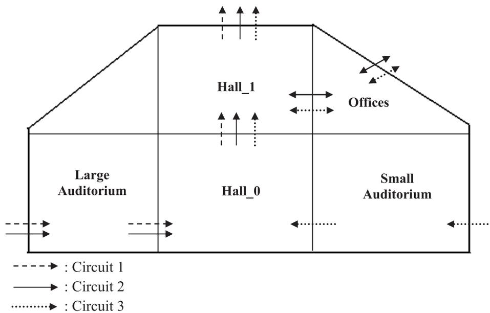
Figure 16. Natural ventilation circuits.
