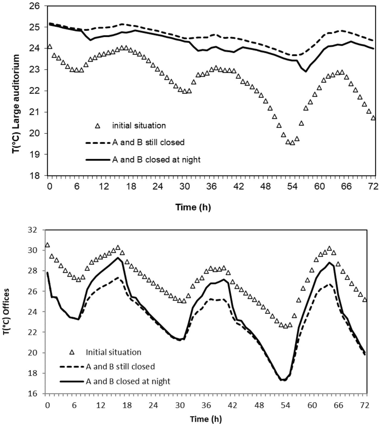
**Figure 13.** Effect of varying flow rate (due to the operating mode of the two valves A and B) in (a) the large auditorium, and (b) the offices - Period from July 23 to 26.
