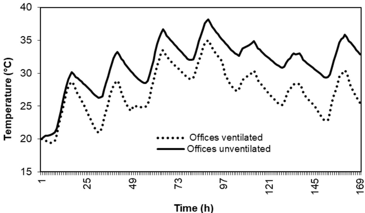
Figure 10. Effect of mechanical ventilation on the offices' temperature during the period of 19 to 26 July.
