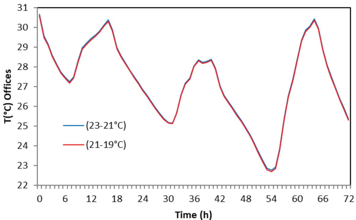
**Figure 11.** Effect of varying ventilation threshold on the offices' temperature.
