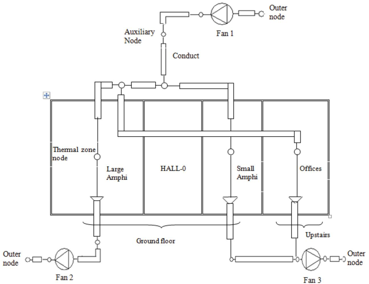
Figure 15. Simple model of the mechanical ventilation circuit that supplies the offices and the two auditoriums.
