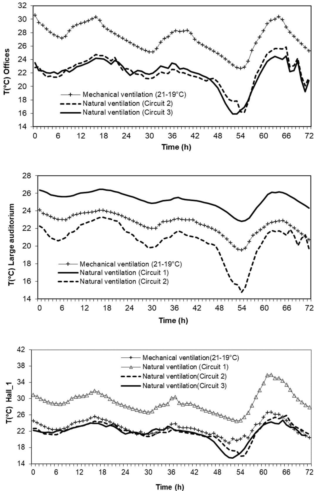
**Figure 17.** Comparison of natural and mechanical ventilation and its effects on the temperature in (a) the offices, (b) the large auditorium, and (c) the Hall\_1.
