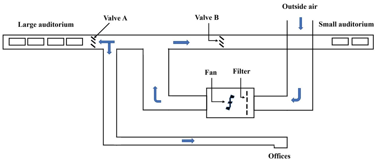
Figure 7. Diagram illustrating the direction of outdoor air conditioning in the building.
