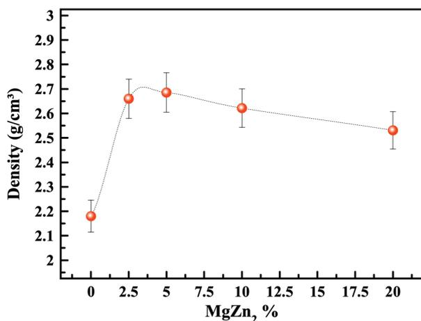
**Figure 1.** The density of the sintered Al alloy with different  $\text{MgZn}_2$  contents.
