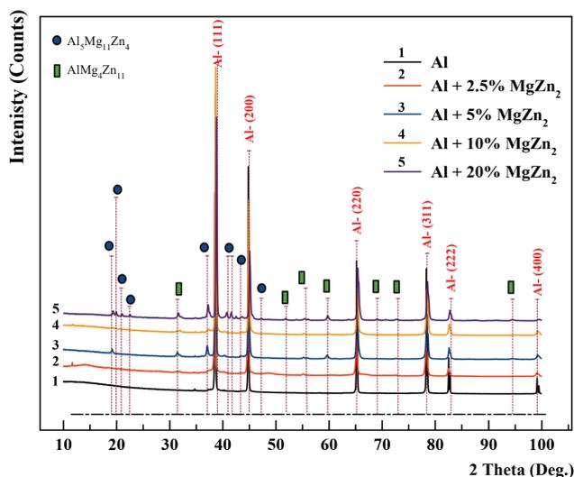
**Figure 5.** XRD diffraction patterns of Al with different MgZn<sub>2</sub> contents.
