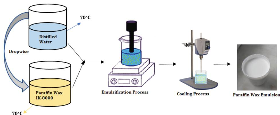
**Figure 1.** Flow Sheet of Paraffin Wax Emulsion Preparation.
