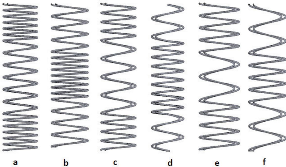
**Figure 2.** Various models of double heat exchanger a) P-2P-P at P=20mm, b) 2P-P-2P at P= 20mm, c) P-2P-P at P= 30mm, d) 2P-P-2P at P= 30mm, e) P-2P-P at P= 40 mm, f) 2P-P-2P at P= 40mm
