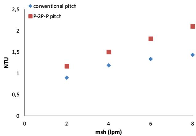
Figure 14. NTU of two double-helical coil models.
