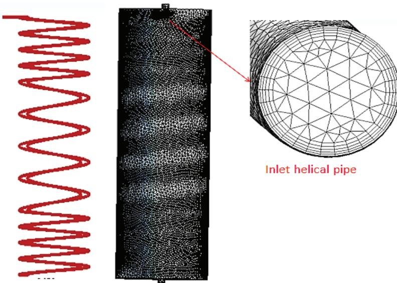
Figure 3. Generated mesh for shell and double coil heat exchanger.
