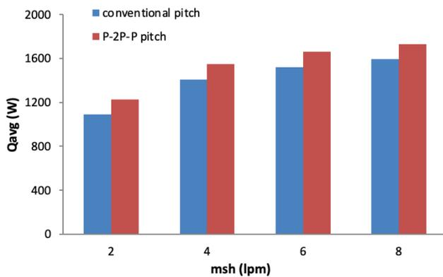
**Figure 10.** Average heat transfer rate variation at different mass flow rate.
