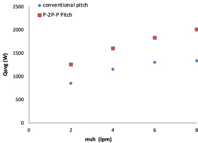
Figure 12. Comparison between average heat transfers rates.
