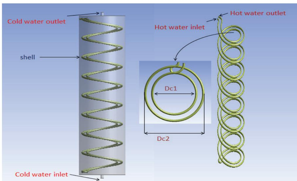
**Figure 1.** Schematic of the shell and double coil tube (baseline case).
