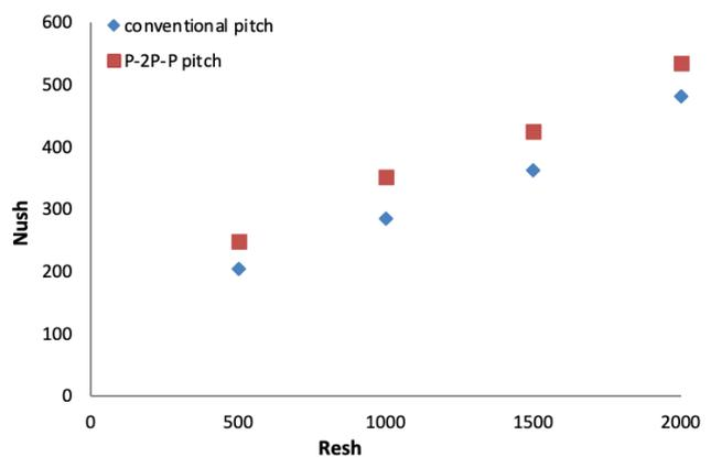
Figure 15. Nusselt numbers of two double-helical coil models.
