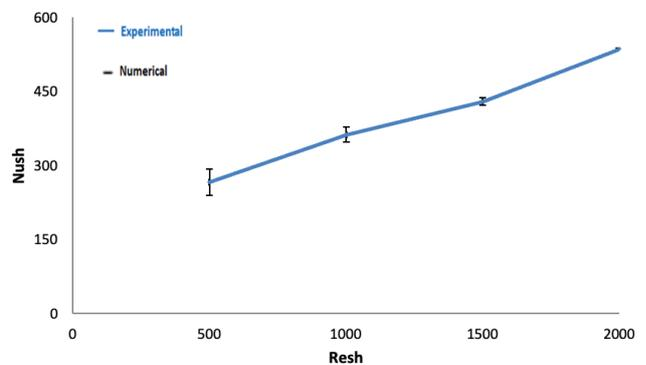
**Figure 11.** A comparison of the numerical simulation and experimental findings for the Nusselt number on the shell side vs. the Reynolds number.
