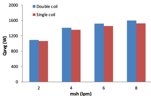
**Figure 7.** Comparison of average heat transfer rate variation for single and double coil at different mass flow rate.
