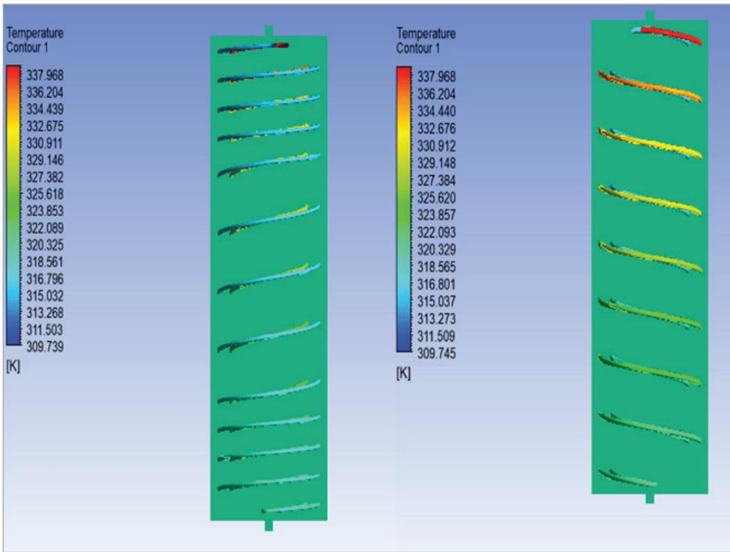
**Figure 9.** Temperature distribution in two models, a double coiled with modified pitch P-2P-P, and conventional pitch heat exchanger.
