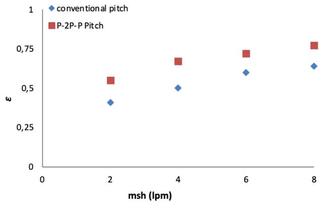
Figure 13. Effectiveness of two double-helical coil models.
