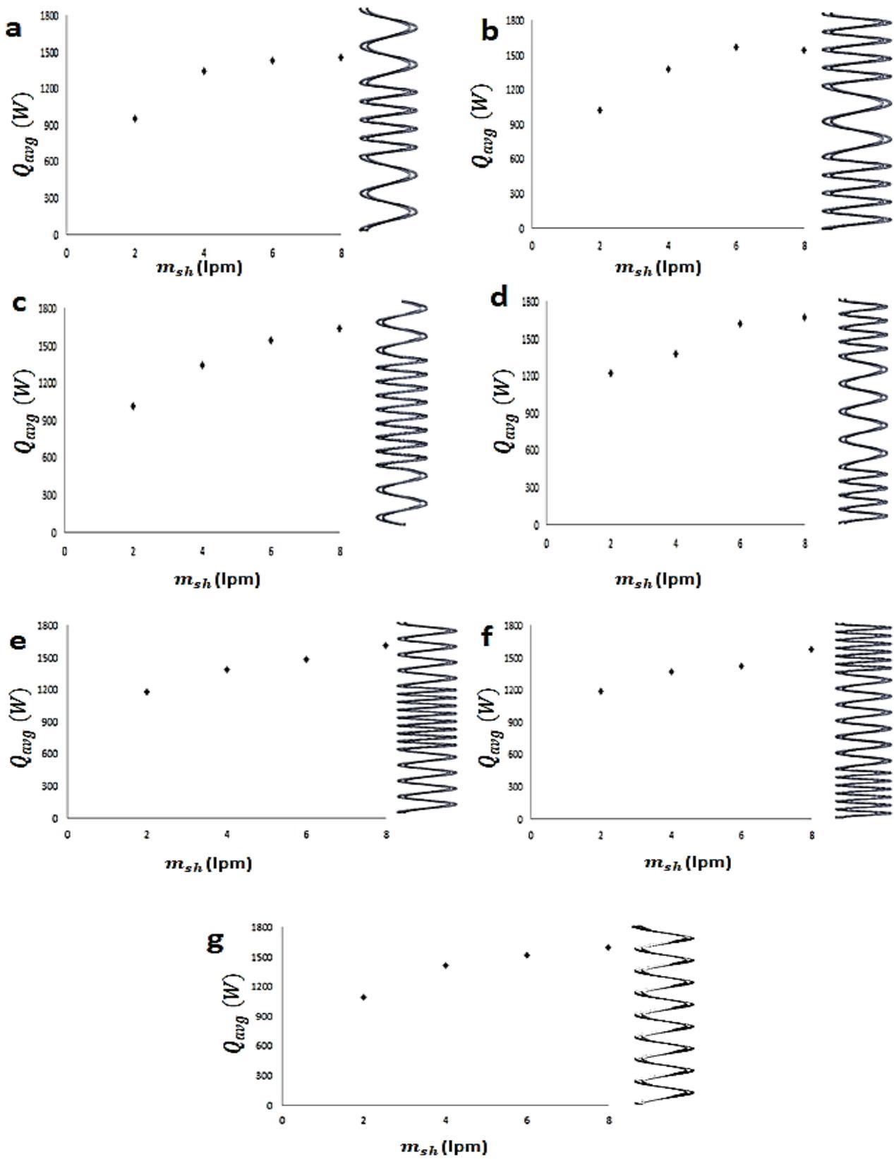
**Figure 8.** Variation of the average heat transfer with coil side Reynolds number 11100. a) 2P-P-2P at P=40mm, b) P-2P-P at P= 40mm, c) 2P-P-2P at P= 30mm, d) P-2P-P at P= 30mm, e) 2P-P-2P at P= 20 mm, f) P-2P-P at P= 20mm, g) conventional pitch.
