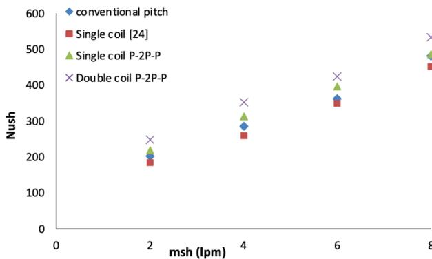
**Figure 16.** The Nusselt number for the shell side compared between the four models.
