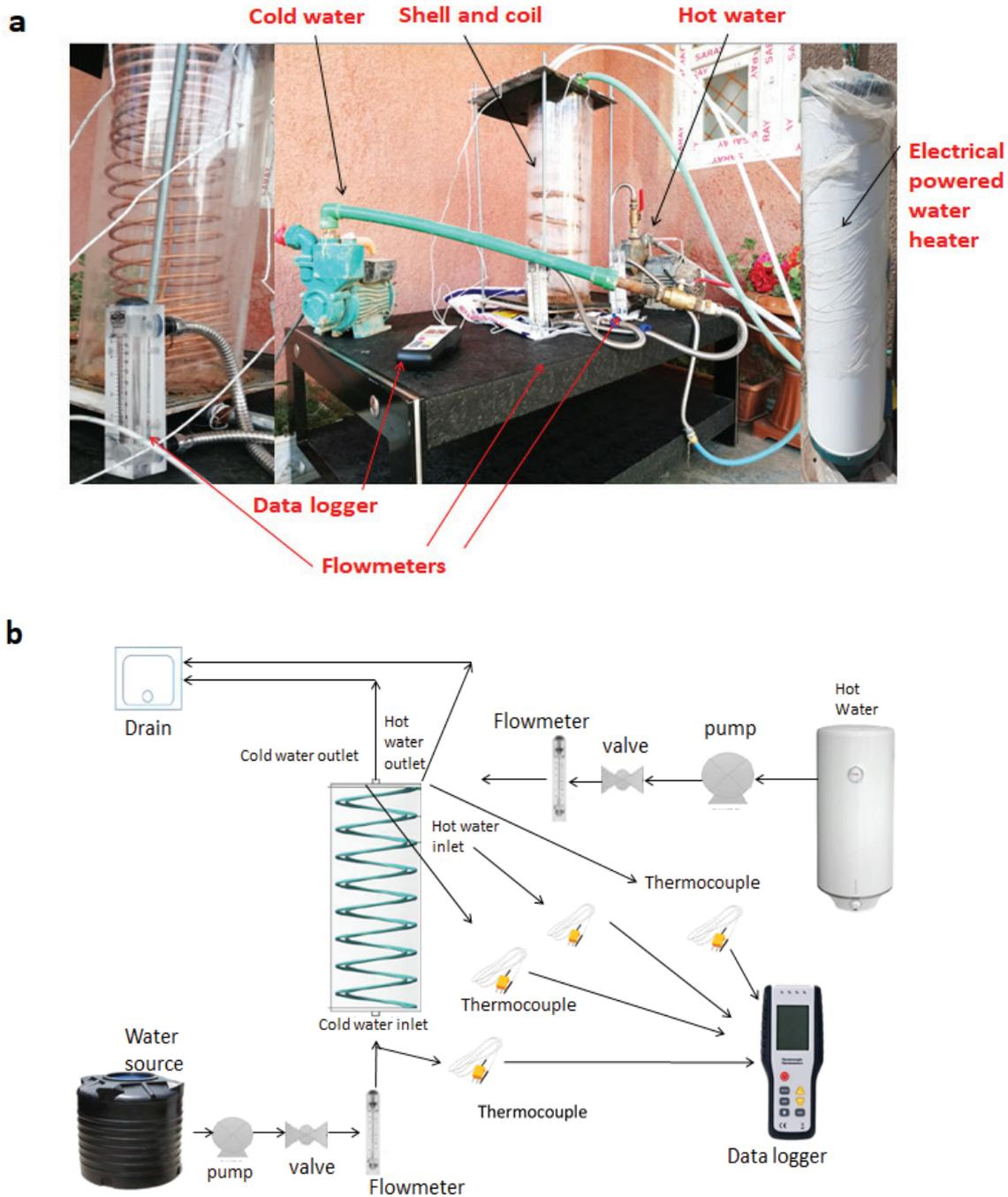
**Figure 4.** a) Image setup experimental work of double coil, b) Schematic diagram of the experimental set up.
