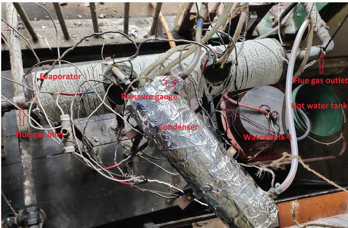
Figure 3. Photograph of experimental system.
